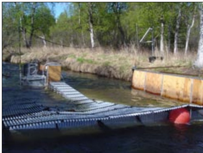
FIGURE 6. — Video monitoring chute, Nikolai Creek, Alaska. Fish passing through the passage chute swim through a video chamber, where they are filmed. Fish can be counted by viewing the video tape in the office.
