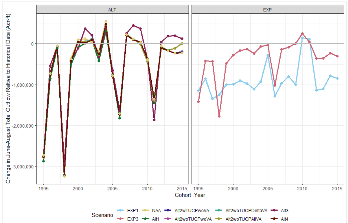
Figure F.1-2. Difference in June-August Total Outflow relative to observed data used for model fitting.
