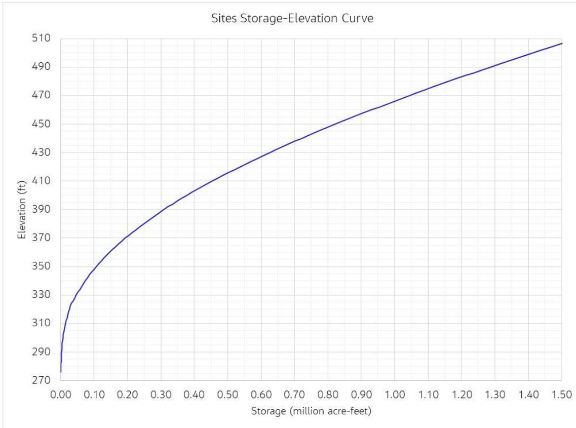
**Figure 6D-2. Sites Storage-Elevation Curve**
