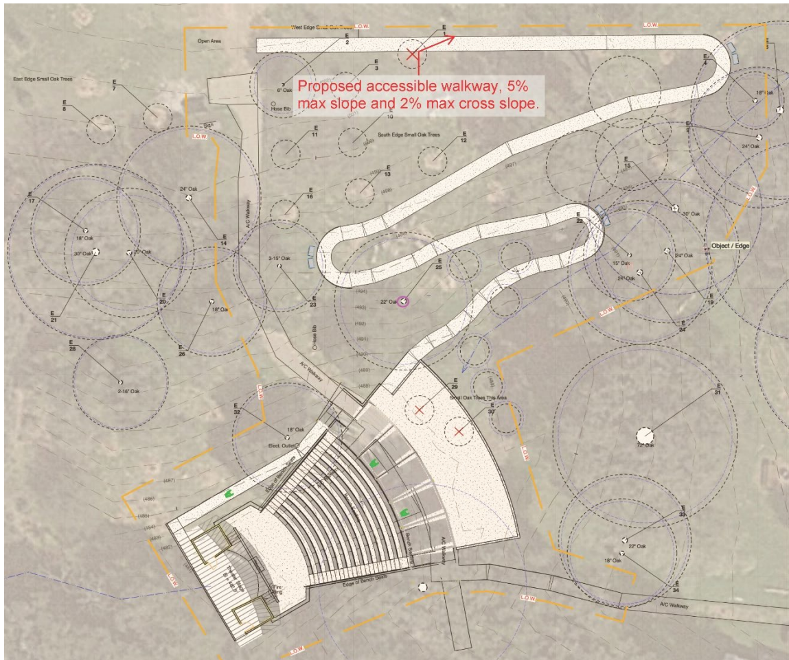
Figure 5. ADA-Accessible Amphitheater Walkway Design Plans
