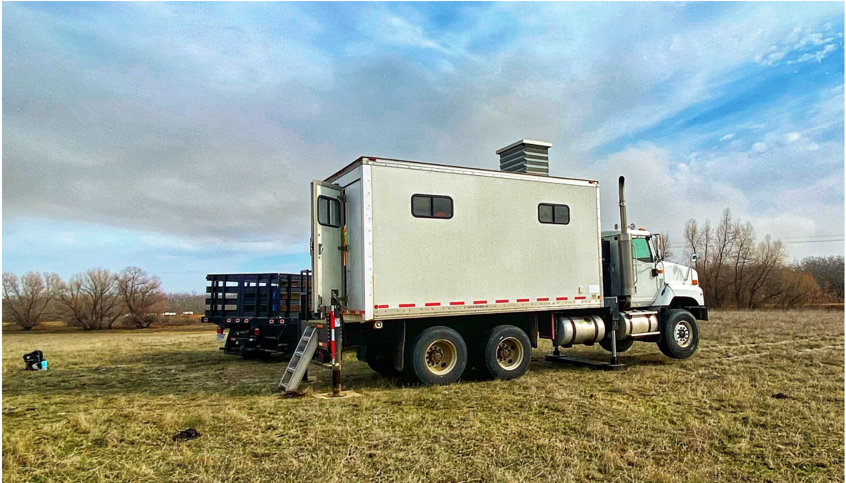
Photo 3 – Representative photo of CPT in grass field
