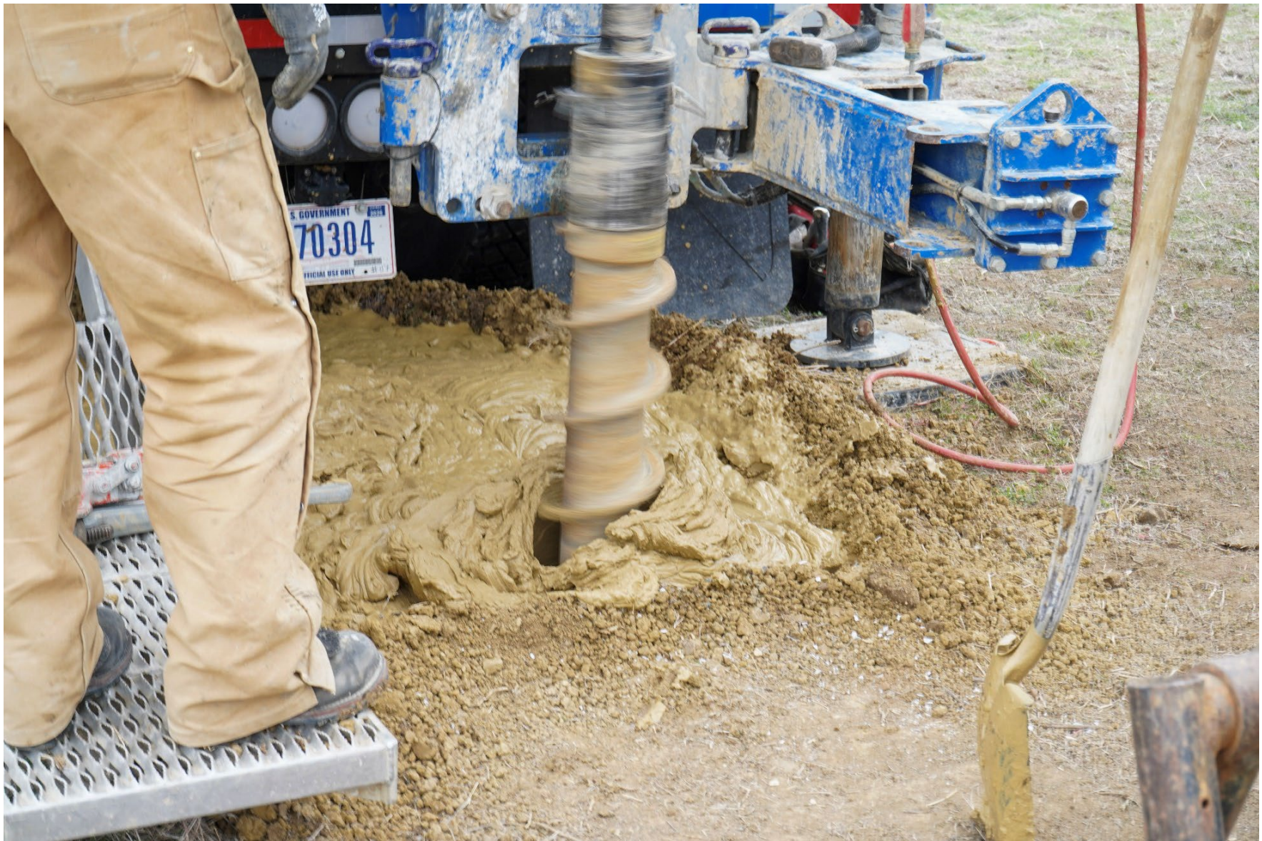
Photo 4 – Representative photo of rotary auger boring.
