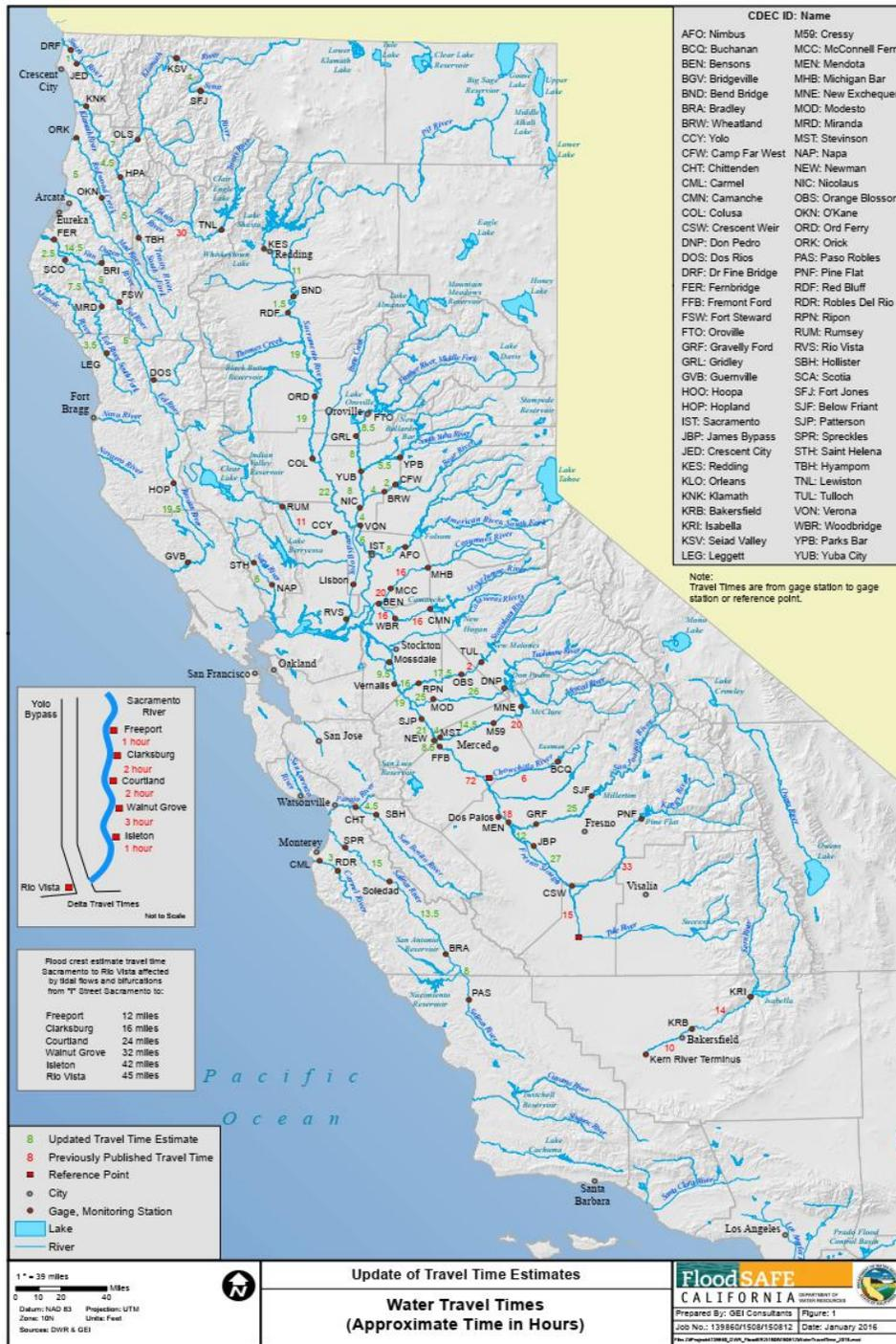
Figure 5A7-3. Water Travel Times (in hours) between gage stations or reference points (GEI Consultants, 2016).
