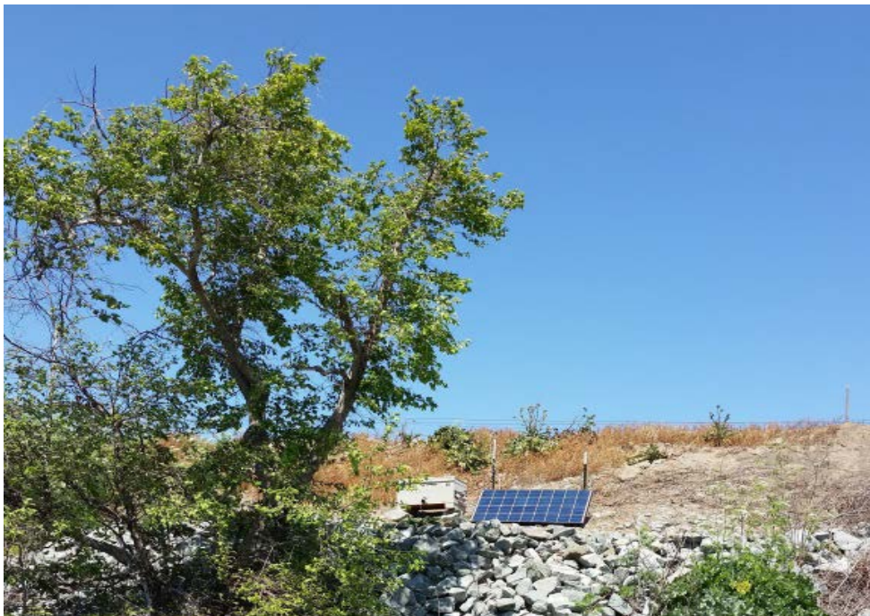
Figure 15: Receiver Site with Datalogger and Solar Panel Located at Grant Line Canal (GL1)
