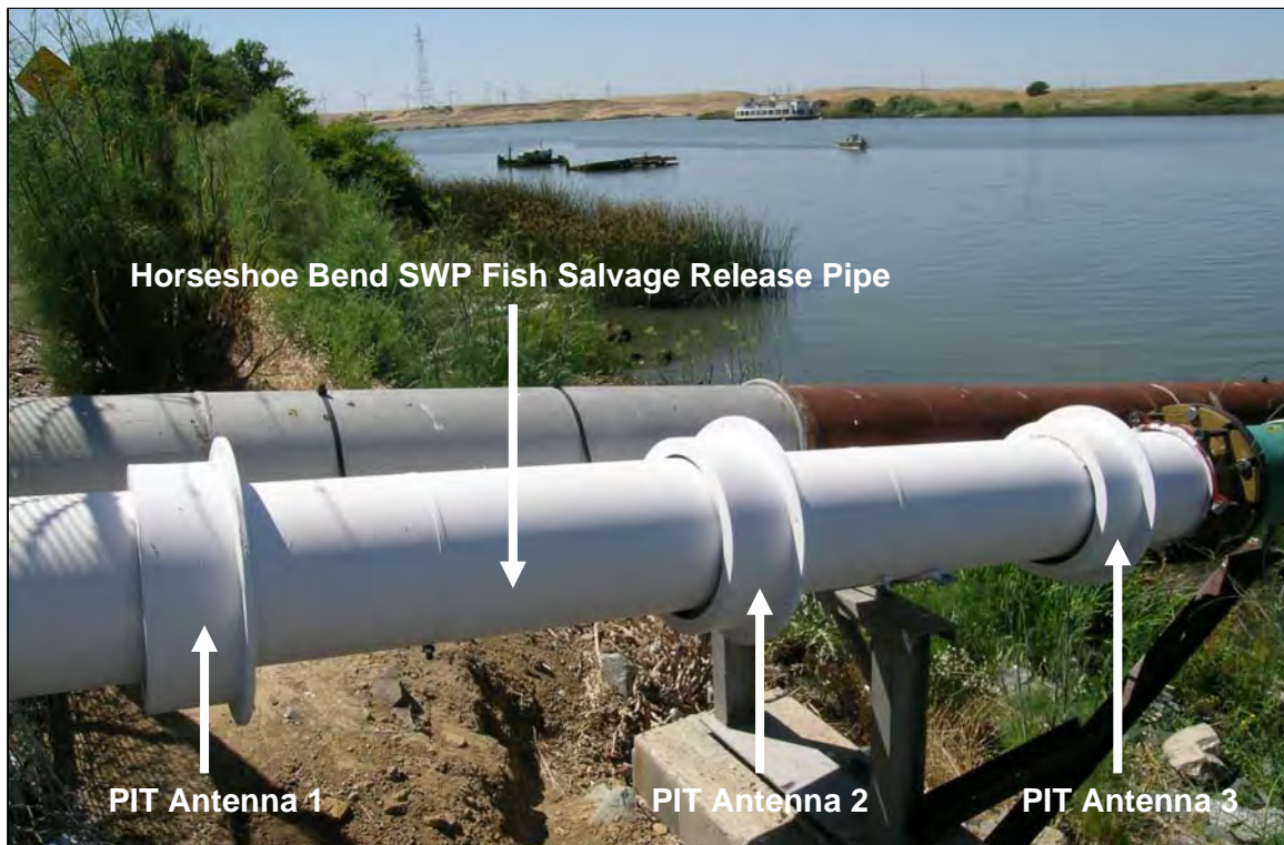
Figure 37. PIT antennae installed around the release pipe at the Horseshoe Bend, SFPF salvage release site.
