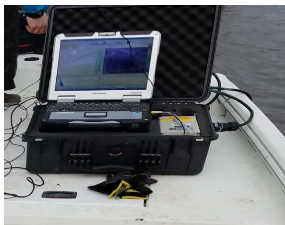
Figure 17: Mobile Datalogger and Laptop Unit and Hydrophone Attachment on Boat
