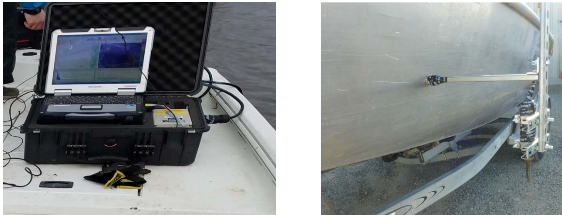
Figure 18: Mobile Datalogger Unit and Hydrophone Attachment
