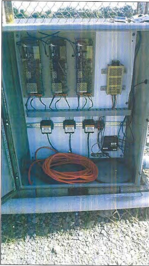
Figure 1- PIT tag detection array installed at the Horseshoe Bend Release Site. Shown are the three Biomark IS1001 transceivers/dataloggers (left) and three custom antennas with their aluminum shields mounted on the salvage release pipe (right).
