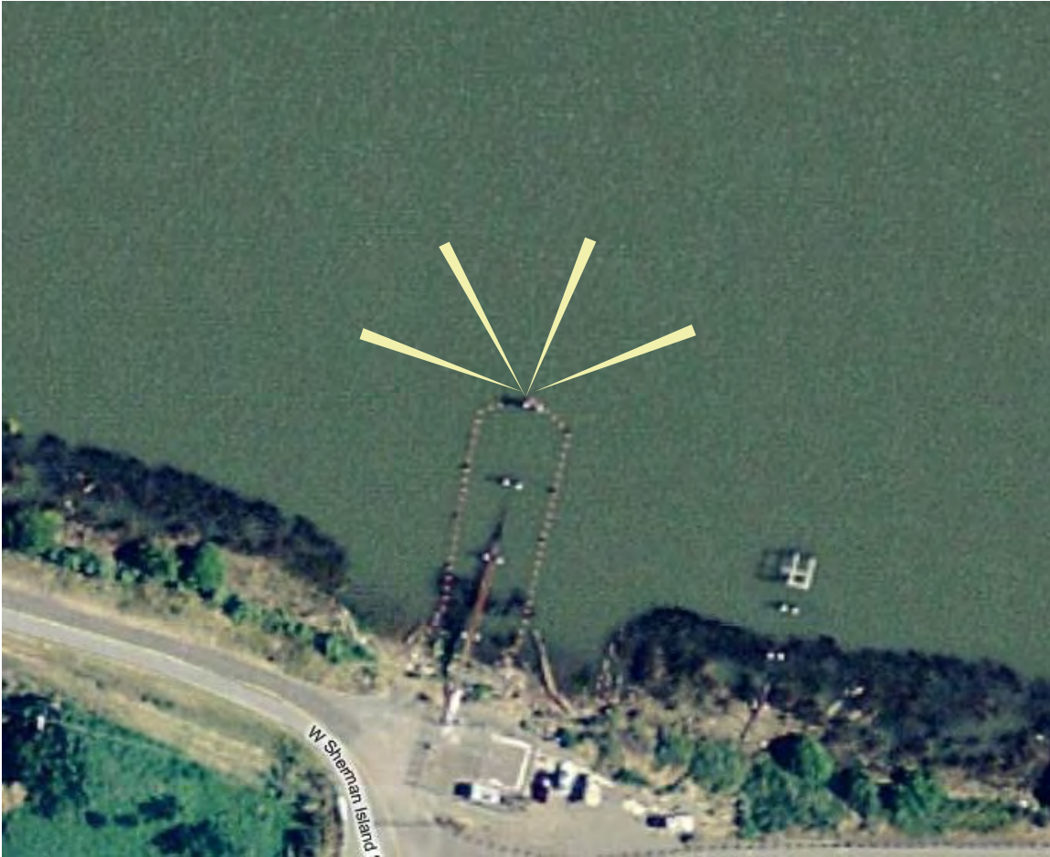
Figure 35- Location of four transducer beams as they sample near the outlet pipe location. Beams and beam spreads are approximately to scale, with a range of 25 m (82 ft) and a beam angle of 6.5^\circ .
