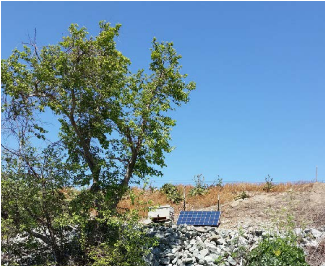
Figure 16: Deployed Model 395 Datalogger/Hydrophone Unit with Solar Panel
