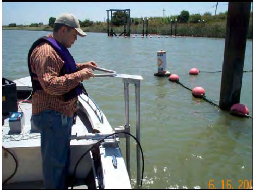
Figure 26- The DIDSON being used for mobile monitoring. The direction that the camera was pointed could be manipulated using the handle bars shown in the photo.
