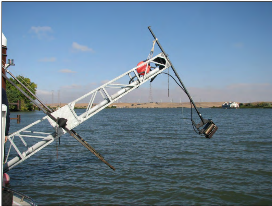
Figure 23- The fixed mount system being lowered into the water at the SWP Horseshoe Bend release site. Note the DIDSON camera at the end of the mount.
