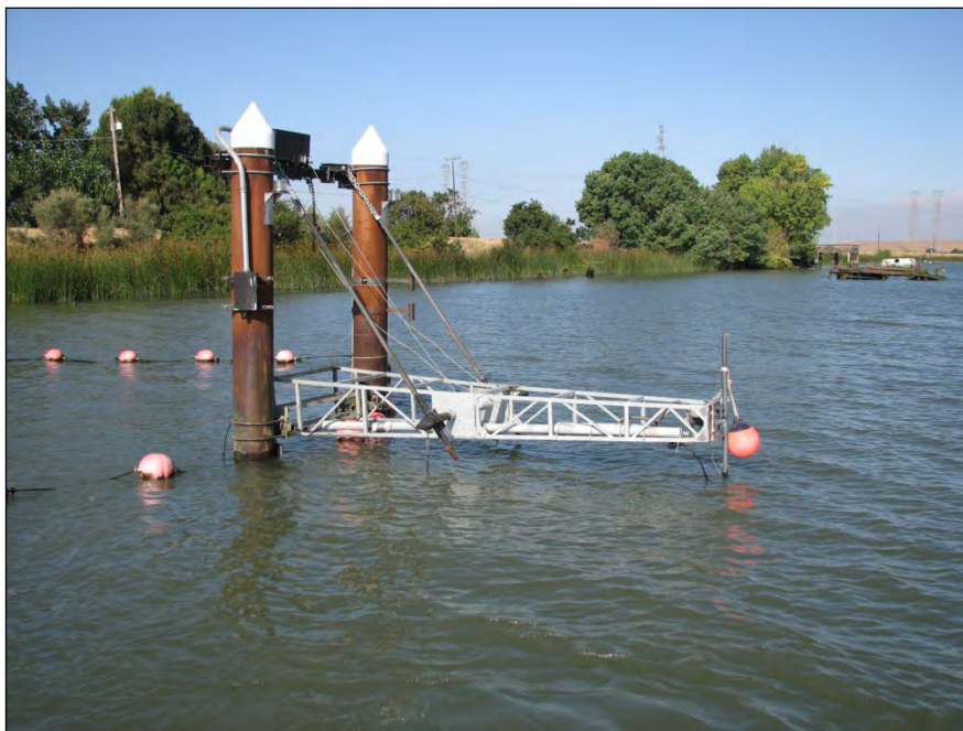
Figure 24- The DIDSON camera mount system in its fully deployed position.
