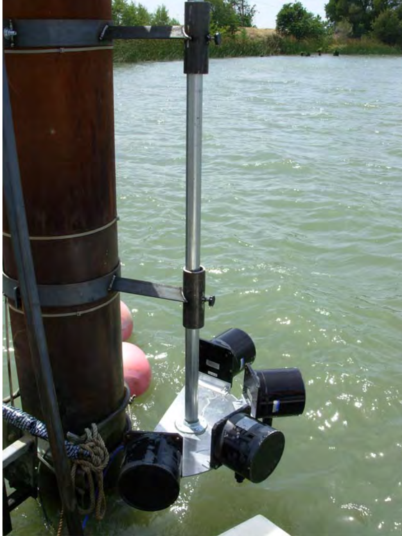
Figure 36- The four-transducer assembly used for this study. The knobs on the mounting brackets could loosen to allow assembly to be raised and lowered. The transducer on the left points almost directly in front of the release pipe. This picture was taken before attaching shore cables to each transducer.
