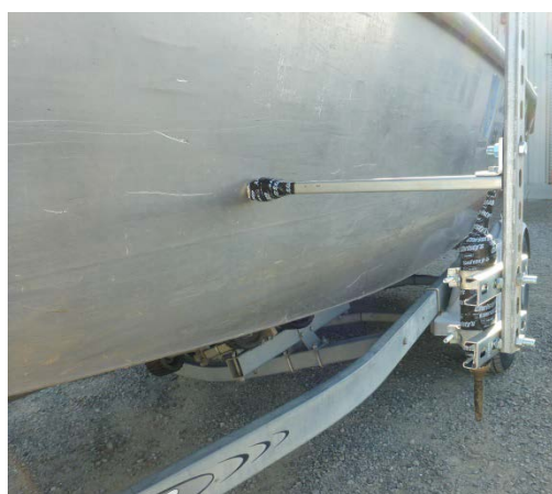
Figure 17: Mobile Datalogger and Laptop Unit and Hydrophone Attachment on Boat
