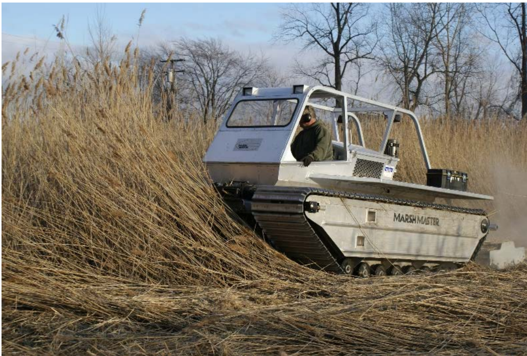
Figure 3. Example of a type of amphibious mower that could be used for the Proposed Action. The specific mower/sprayer combination that will be used is to be determined based on contracting components and needs. Source: https://www.marshmaster.com/
