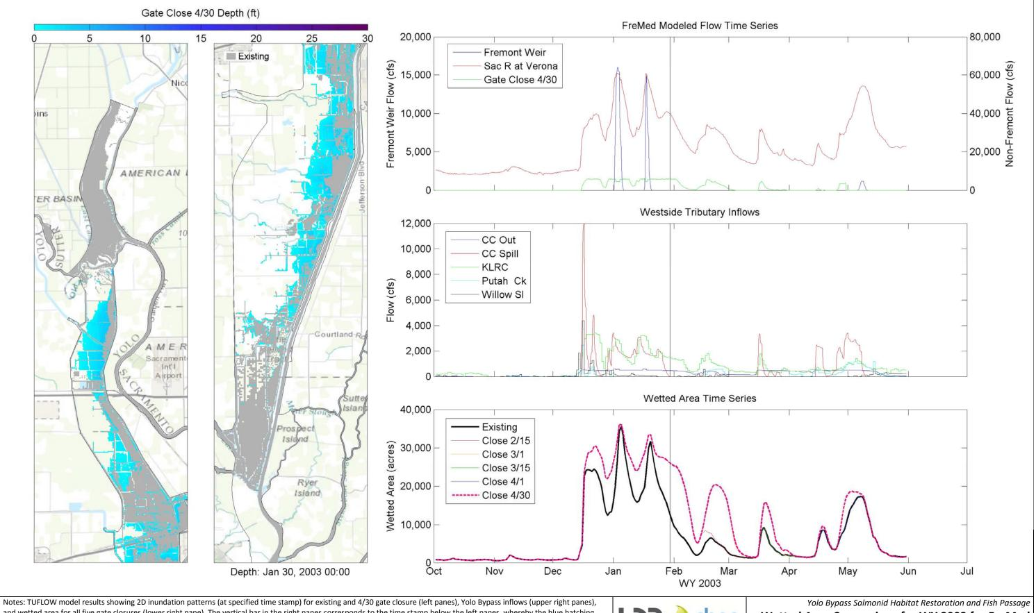
Notes: TUFLOW model results showing 2D inundation patterns (at specified time stamp) for existing and 4/30 gate closure (left panes), Yolo Bypass inflows (upper right panes), and wetted area for all five gate closures (lower right pane). The vertical bar in the right panes corresponds to the time stamp below the left panes, whereby the blue hatching represents 4/30 gate closure conditions as overlain by the grey hatching representing existing conditions.
