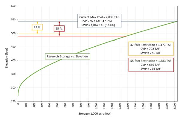
Figure 1-1. San Luis Reservoir Storage vs. Elevation with Restriction Alternatives
