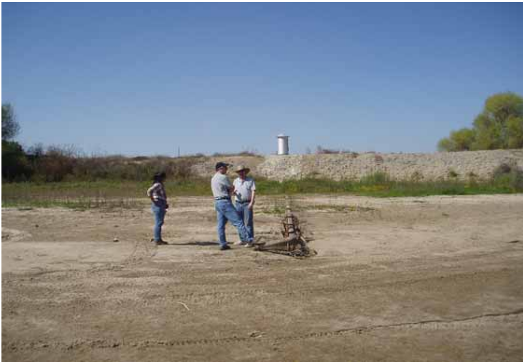
Figure 3: Existing stream gage showing communication line in foreground and stilling well structure on top right stream bank in background.
