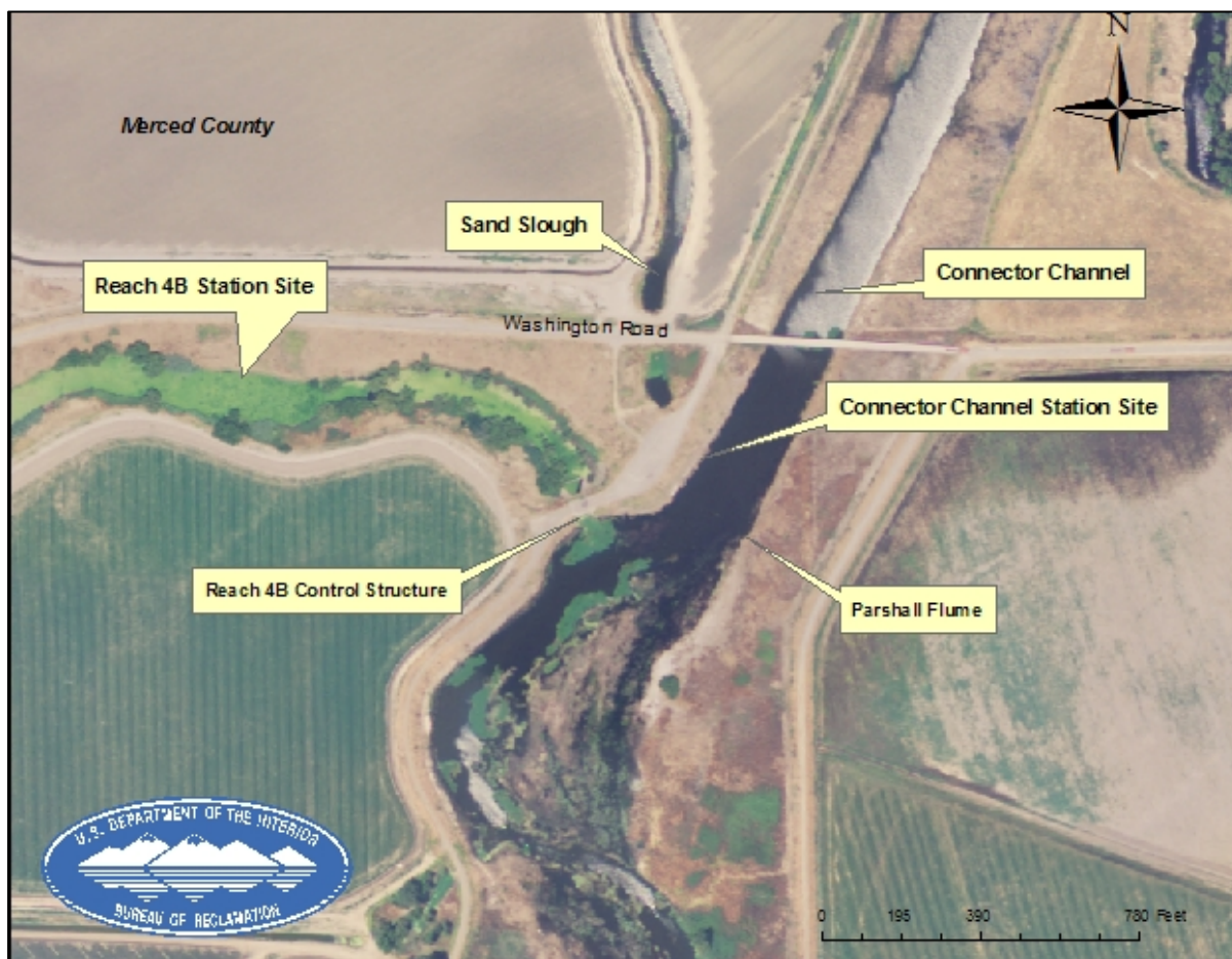
Figure 11: Reach 4B and Connector Channel Flow Monitoring Station Sites.
