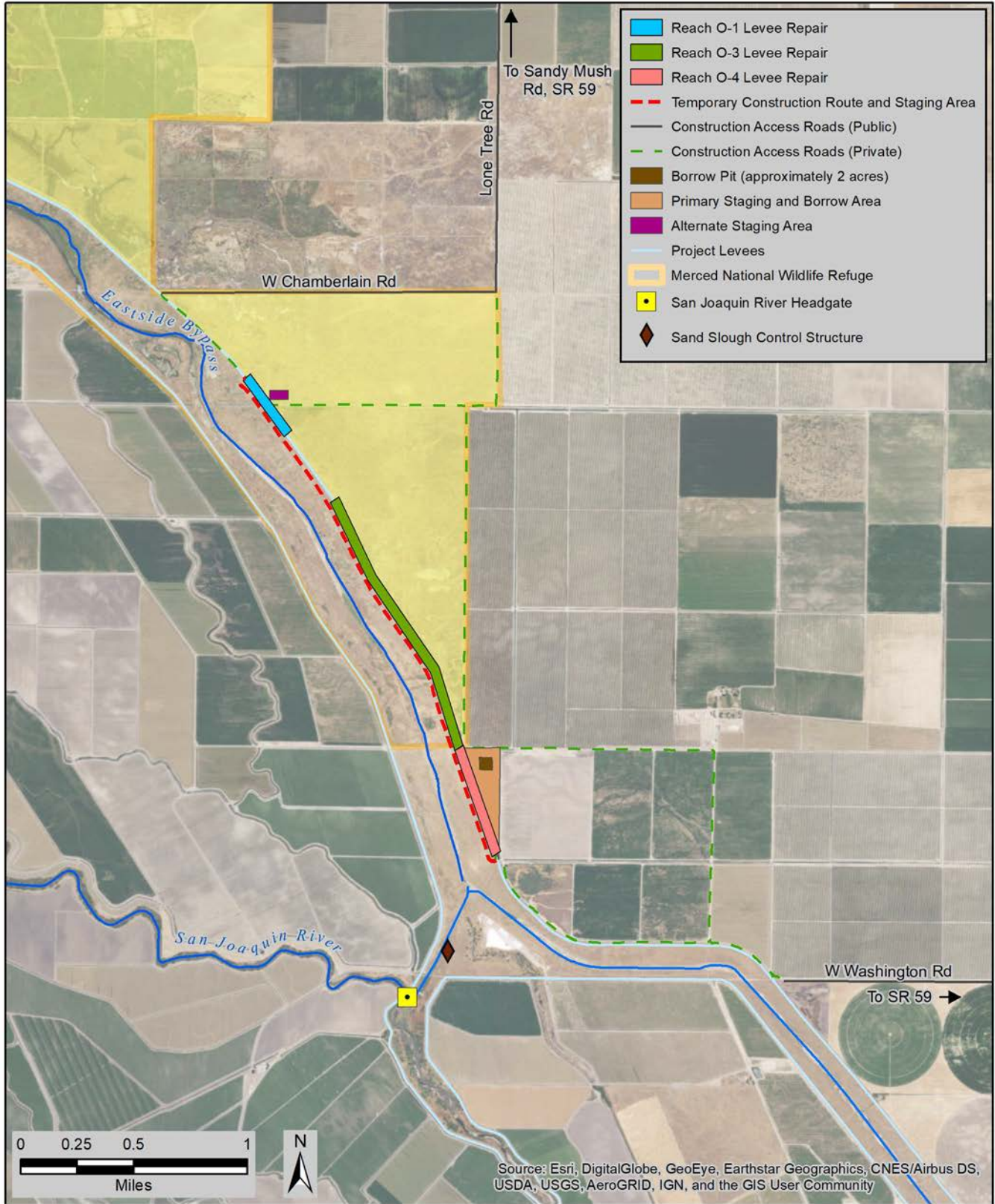
Figure 2-11. Levee Improvement Segments
