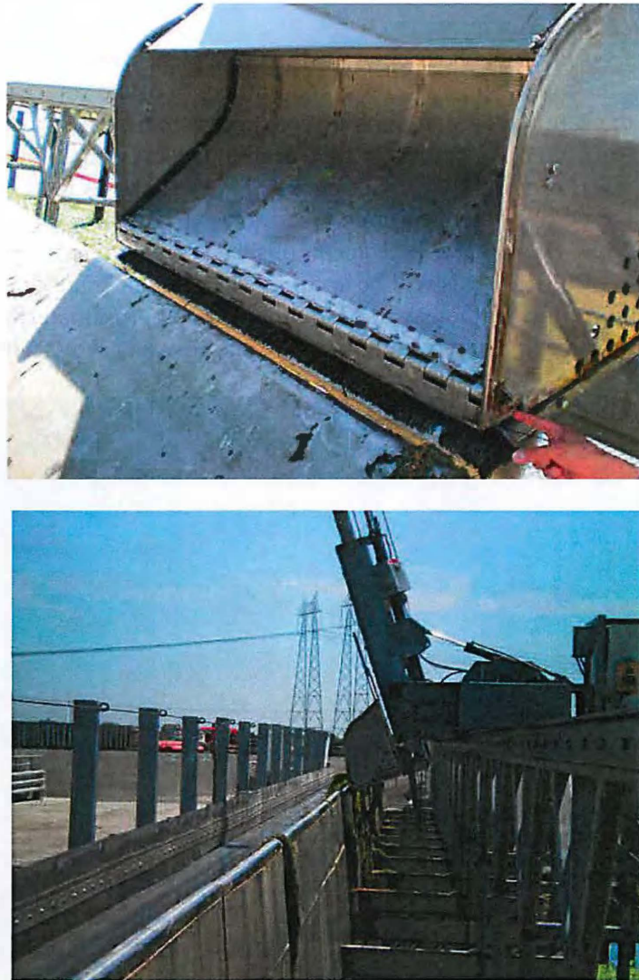
Figure 4. New prototype rake bucket (upper) and hydraulic arm (lower) operating at RSFS (May 29, 2015 site visit).
