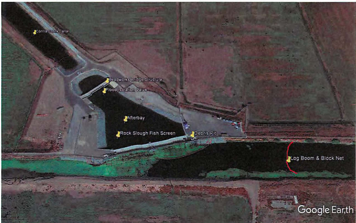
Figure 2. Rock Slough Fish Screen showing facility structures (headworks, afterbay, canal, debris pits), aquatic weeds in 2015, and approximate location of re-located log boom in 2016.
