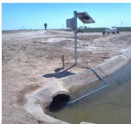
Figure 7. An example of an acoustic/Doppler meter and flow retrofit
