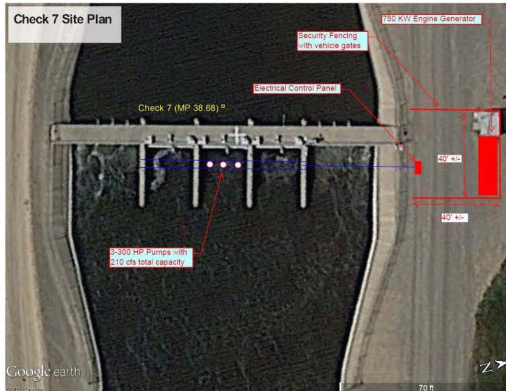
Figure 4 Temporary Lift Station at Check Structure No. 7
