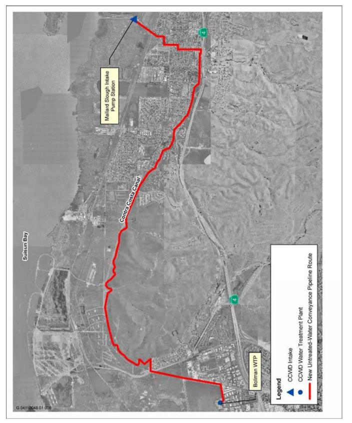
Source: Carollo Engineers Desalination Alternative: Untreated-Water Conveyance Route from Contra Costa Canal Junction to Bollman WTP
