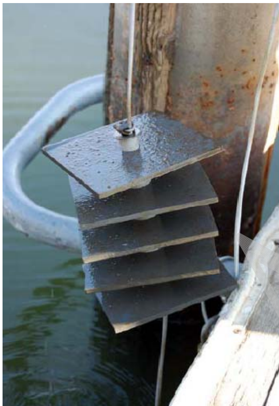
Figure 2. Substrate sampler used for monitoring zebra mussels. Photo Source: CDFG and CA DWR
