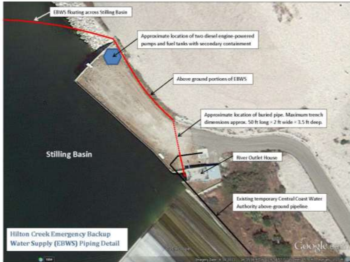
Figure 3 Pipeline Trenching Details
