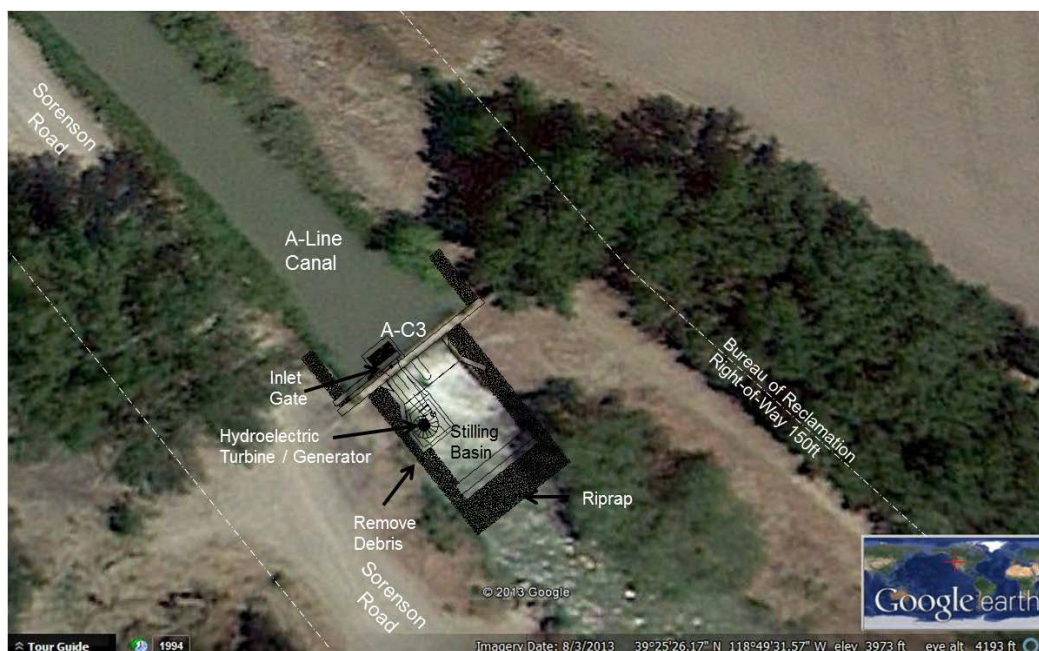
Figure 3 – A-C3 Panicker Drop Check Structure / Hydroelectric-Turbine Location
