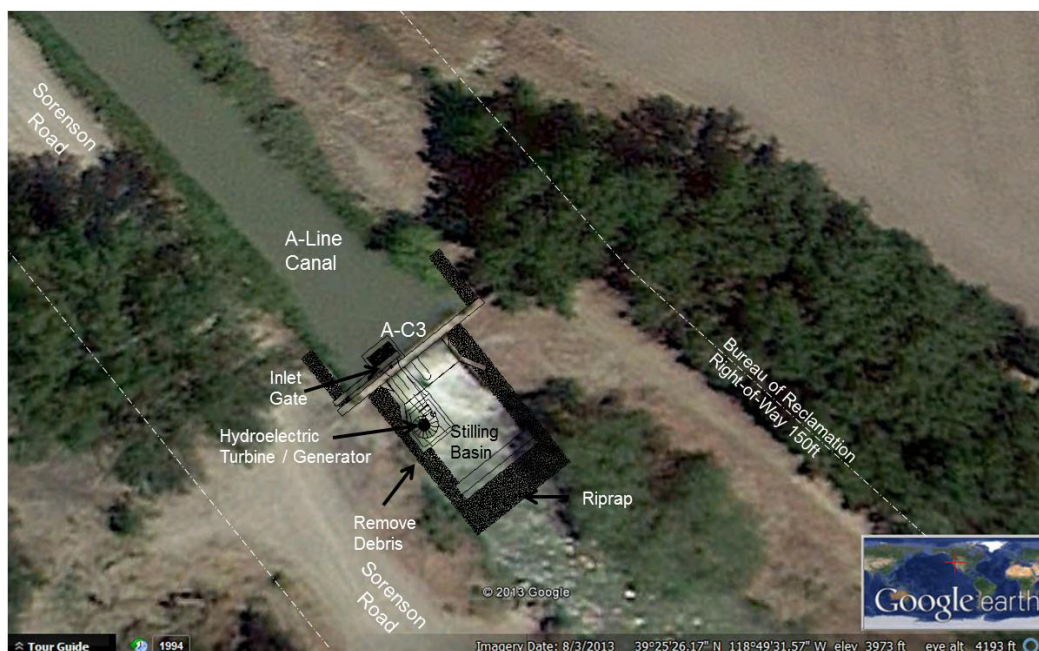
Figure 3 – A-C3 Panicker Drop Check Structure / Hydroelectric-Turbine Location
