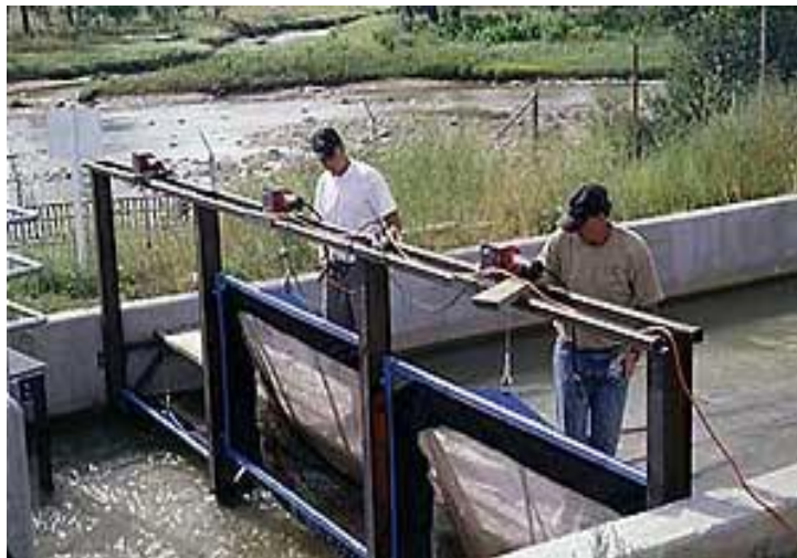
Figure 3. Example Entrainment Netting (Bureau of Reclamation)
