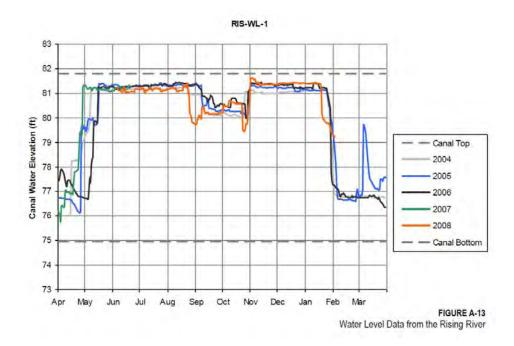
Figure 3 – DDR Figure A-13 showing water level in Rising River (Traynor) Lateral
