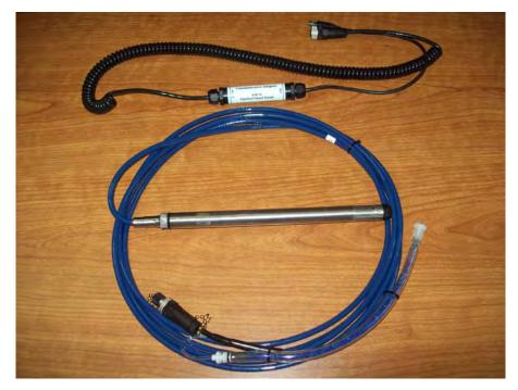
Figure 1 - Instrumentation NW PT2X smart sensor and cable. Source: AW Blair Engineering
