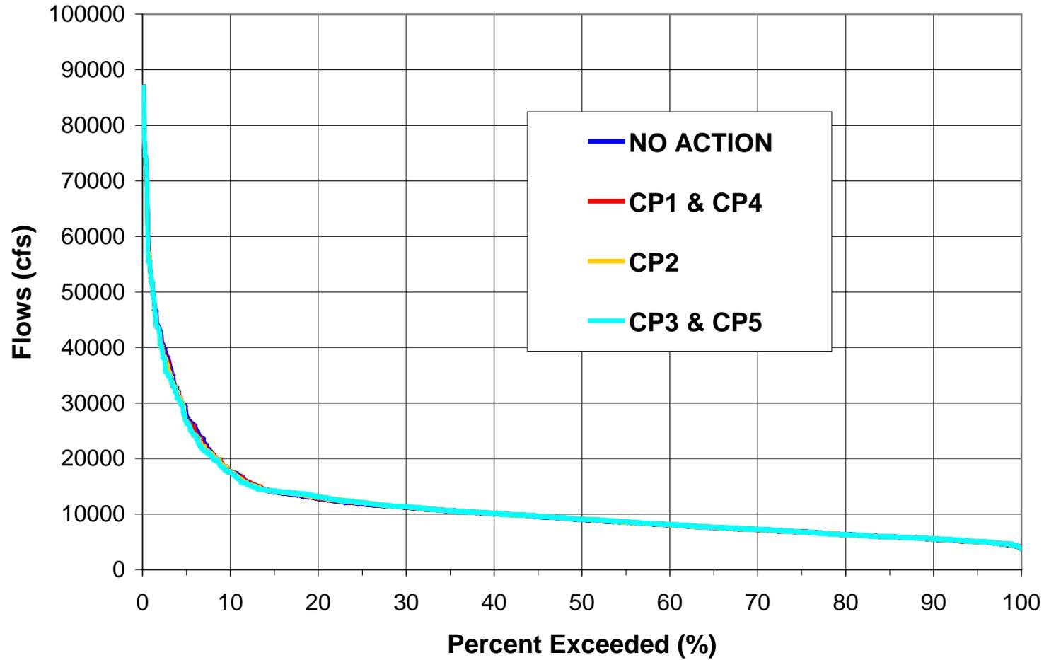
Figure 11. Frequency distribution of monthly flows out of Red Bluff Diversion Dam for the 1921 – 2003 CALSIM period of record.
