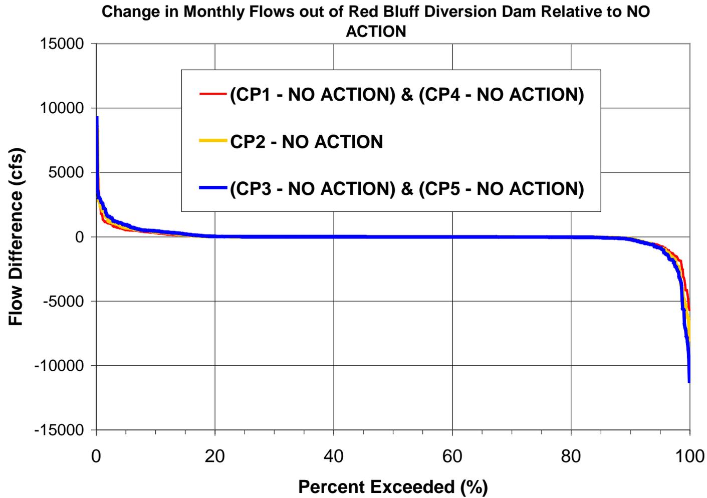
Figure 12. Frequency distribution of change in monthly flows out of Red Bluff Diversion Dam relative to NO ACTION.
