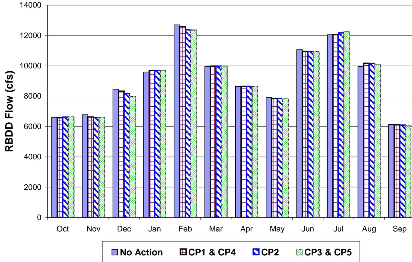
Figure 13D. Average monthly flows out of Red Bluff Diversion Dam (RBDD) during below normal water years.
