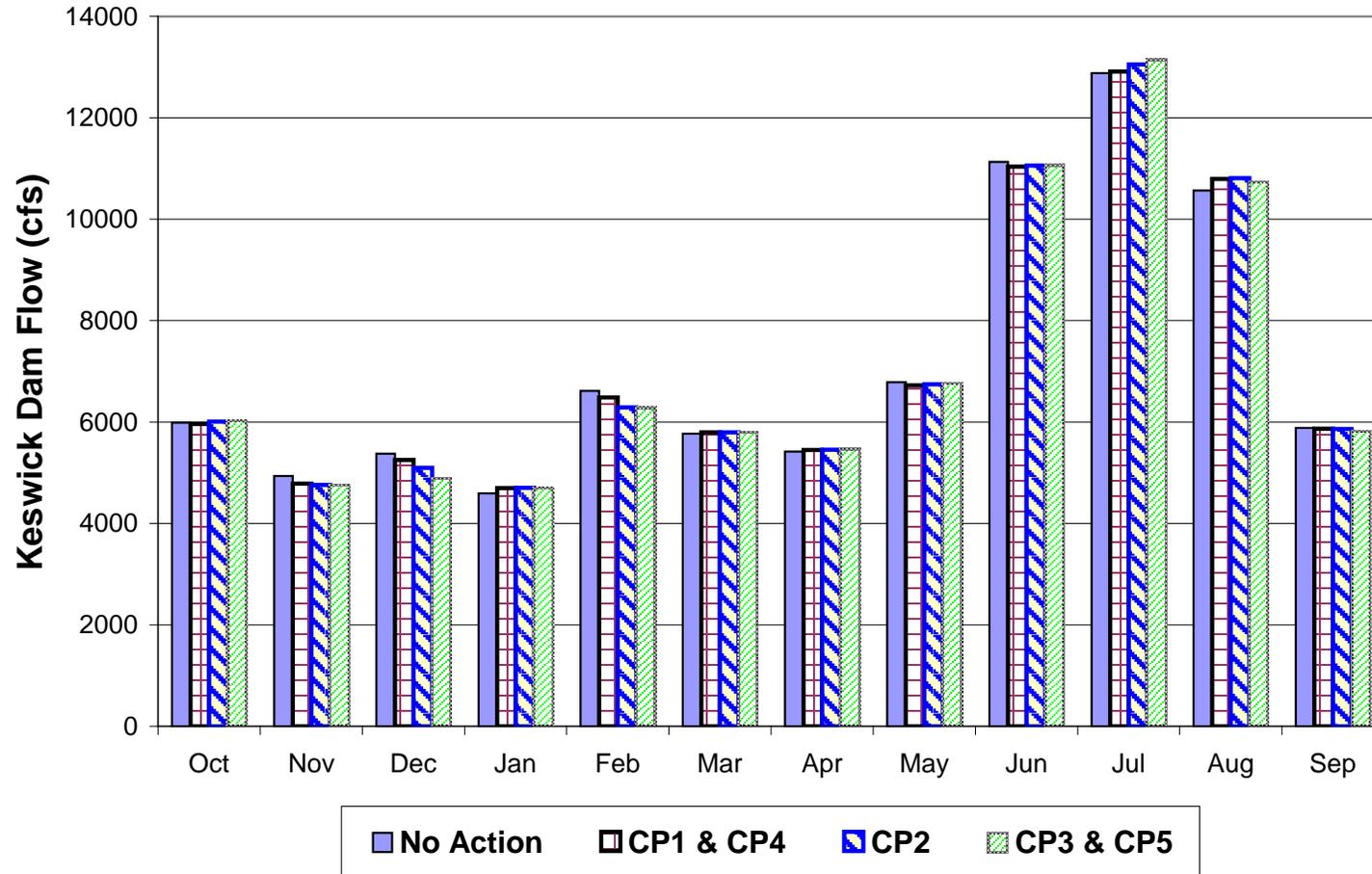
Figure 7D. Average monthly flows out of Keswick Dam during below normal water years for the 1921 – 2003 period of record.
