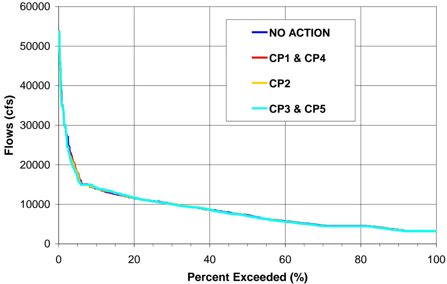
Figure 5. Frequency distribution of monthly flows out of Keswick Dam for the Oct. 1921 – Sept. 2003 CALSIM period of record.
