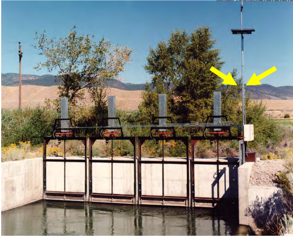
Figure 3 – Water level sensor example showing solar panel and antenna
