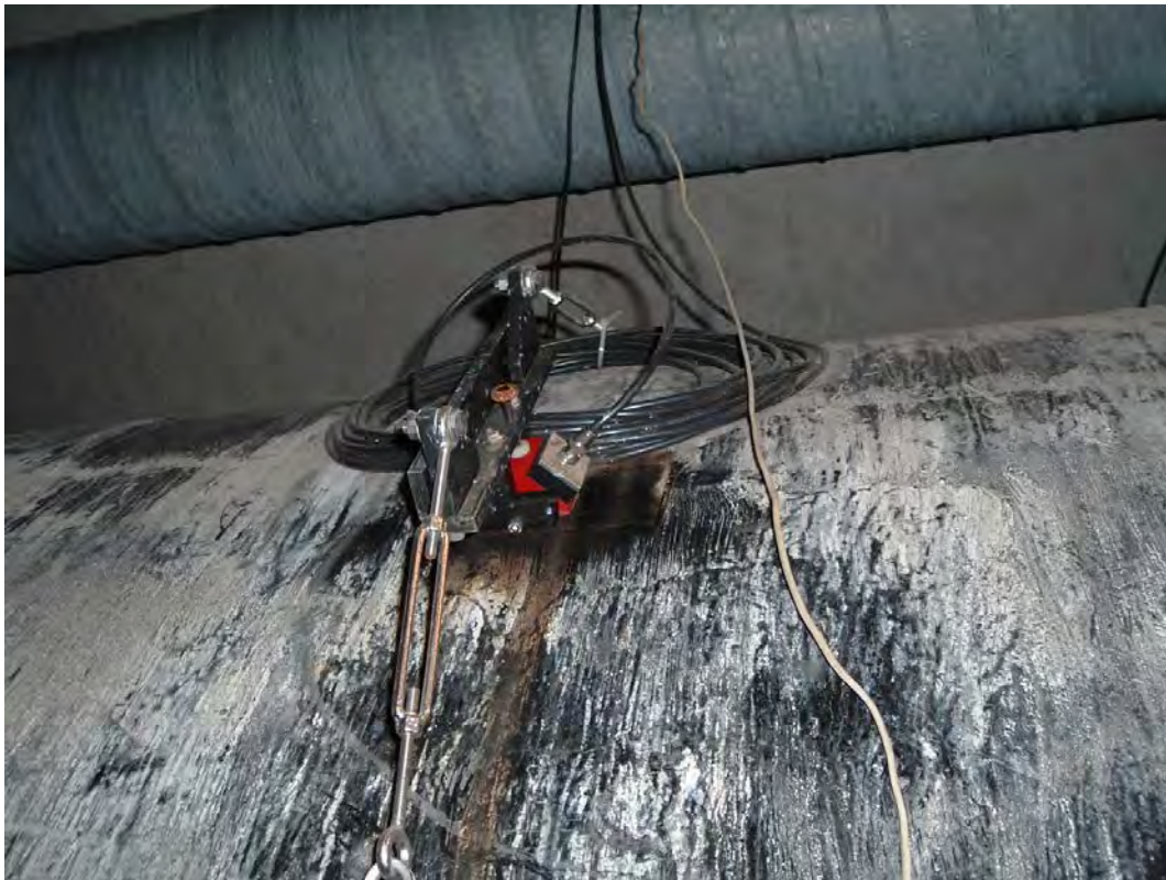
Figure 2 – Example of external flow sensor on penstock pipe
