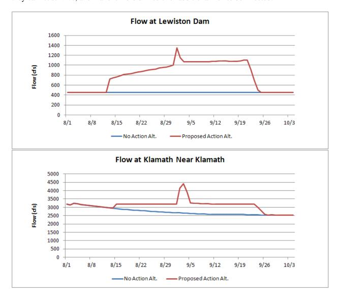
Figure 1. Approximate hydrograph for Lewiston Dam releases to result in the No Action Alternative and Proposed Action preventative flow targets in the lower Klamath River (U.S. Geological Survey Site #11530500: Klamath River near Klamath, California) during the 2012 fall-run Chinook salmon migration period.
