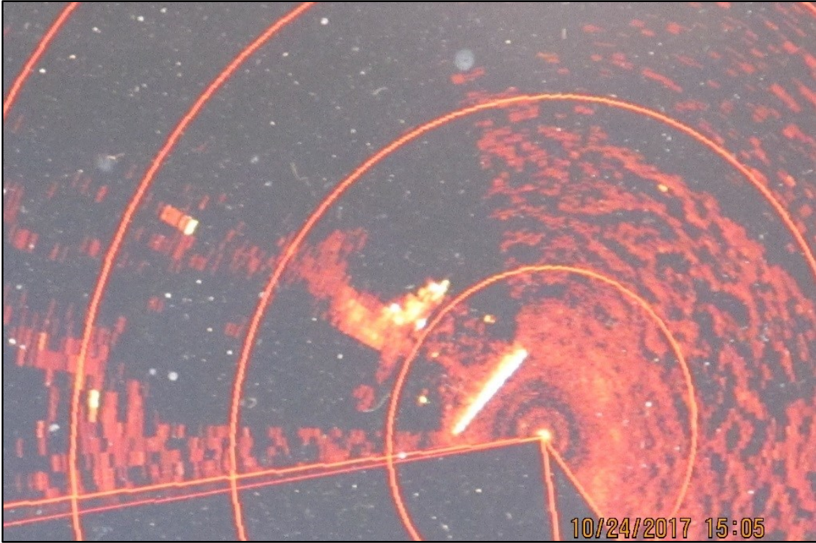
Whiskeytown Lake, Spring Creek Temperature Control Curtain A view of the sector scan sonar unit being used to find the anchor blocks.
