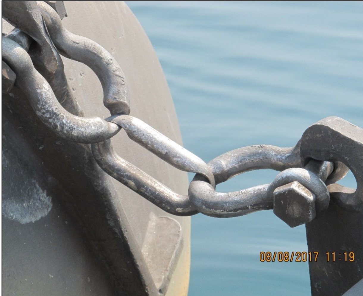
Whiskeytown Lake, Spring Creek Temperature Control Curtain A view of the eroded chain, shackles, and curtain support float ears.
