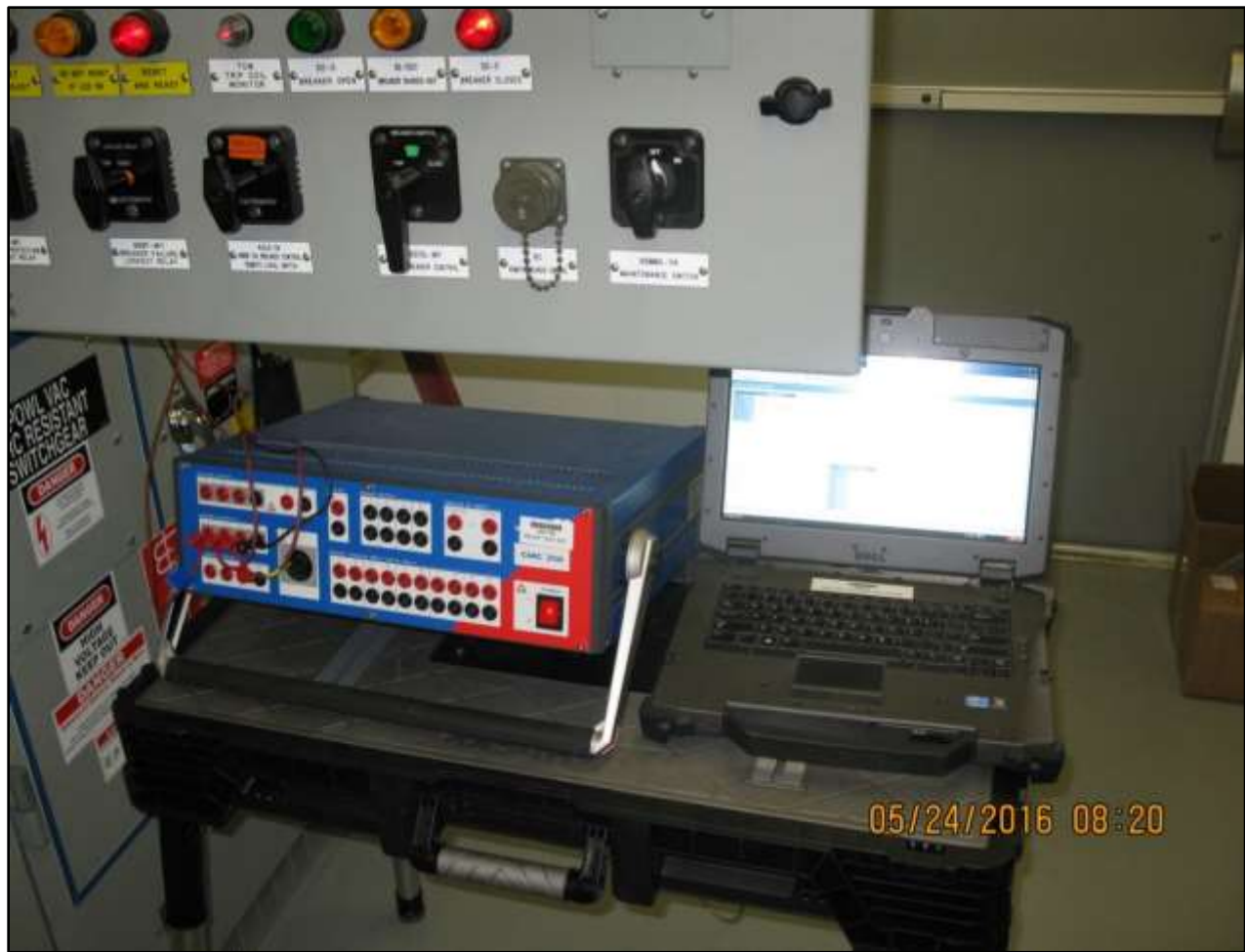
Tracy 13.8kV Switchgear/Break Replacement The Testing equipment used by San Luis and Delta Mendota Water Authority electricians to inject current into the DFR from each breaker.
