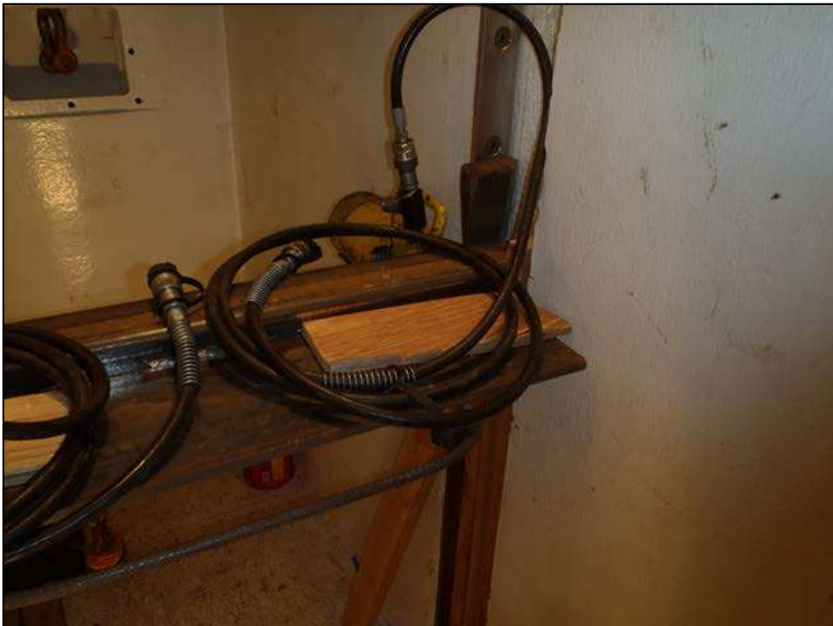
Prosser Creek Dam Refurbish High-Pressure Gate Seats and Regulating Gates A hydraulic jack used to apply force on the gate leaf to check clearances.
