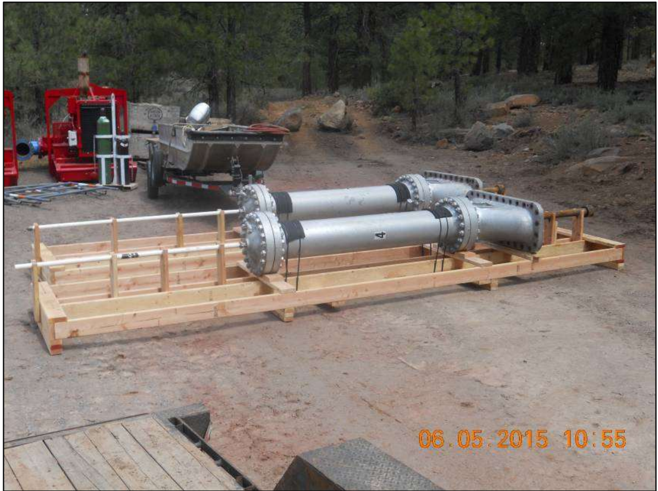
Prosser Creek Dam Refurbish High-Pressure Gate Seats and Regulating Gates Gate Cylinder and Bonnet assemblies ready to be transported
