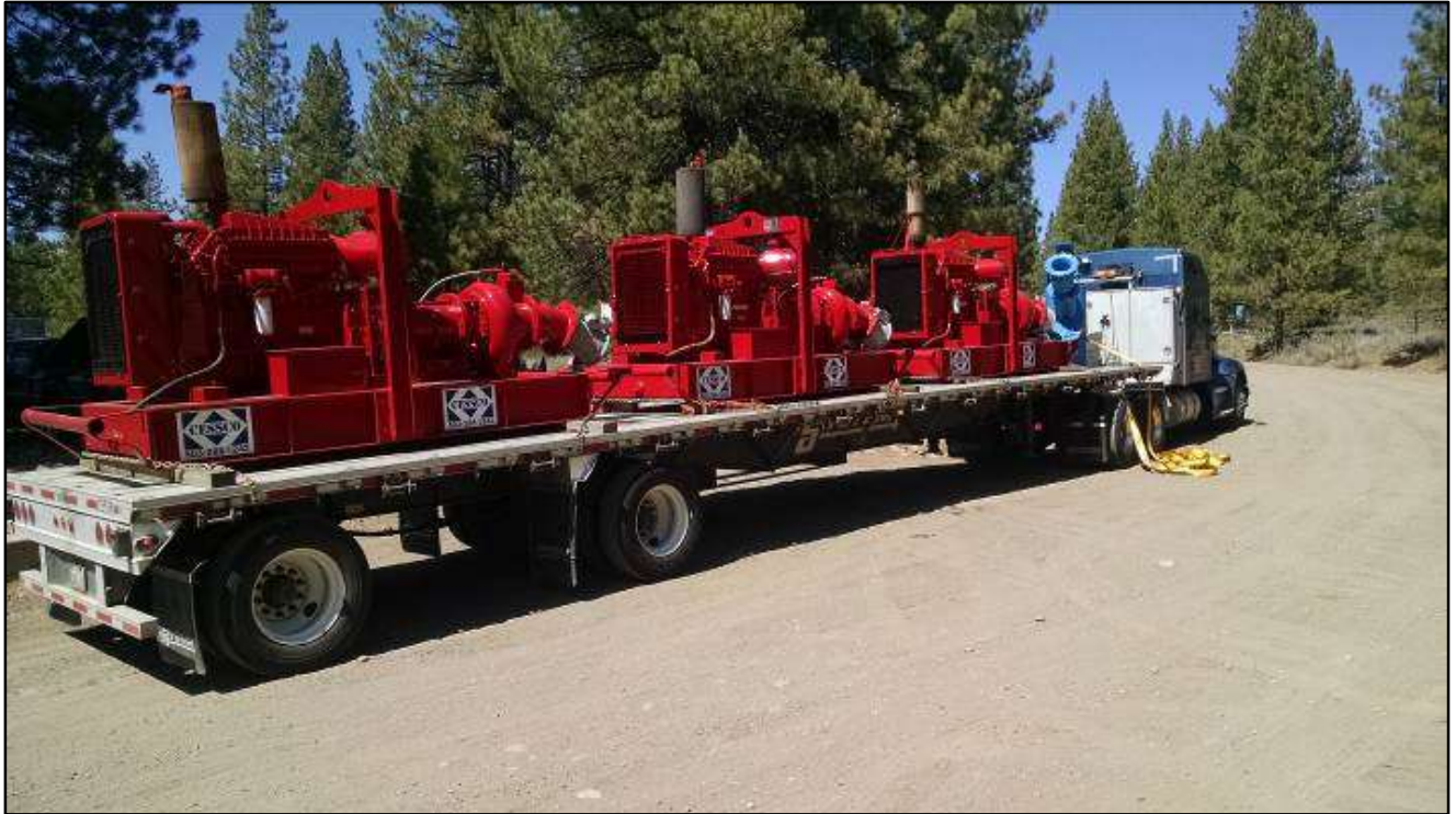
Prosser Creek Dam Refurbish High-Pressure Gate Seats and Regulating Gates Delivery of the three CD300M Diesel water pumps for bypassing water.
