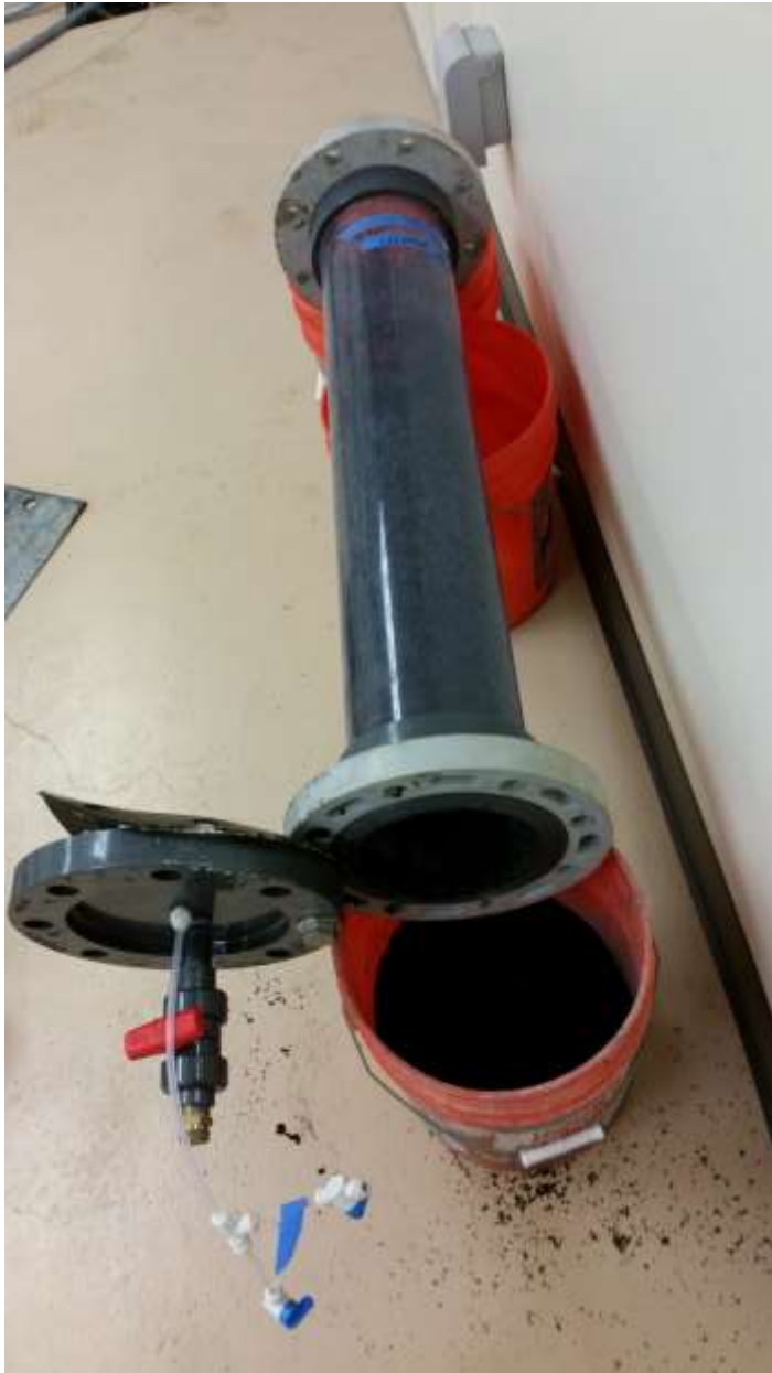
San Luis Demonstration Treatment Plant Granular activated carbon sampling from the column in the Treatment Plant lab.
