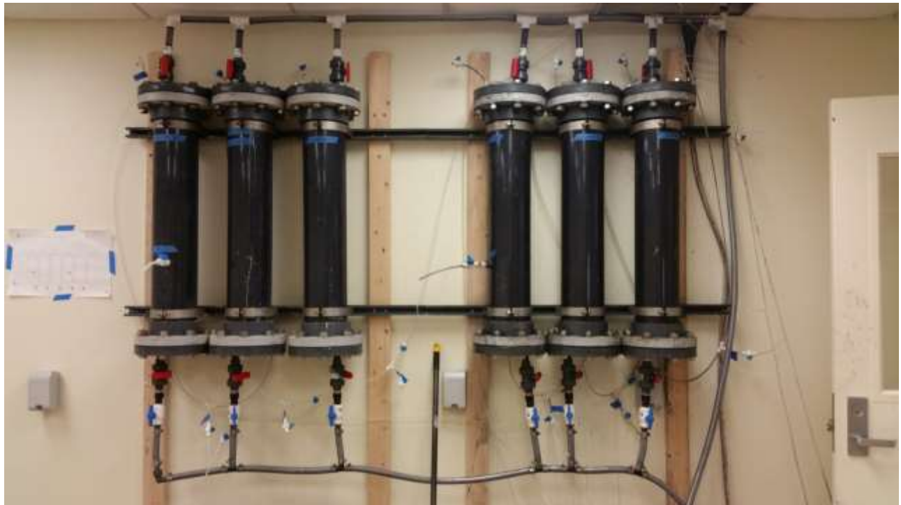
San Luis Demonstration Treatment Plant Photo of the degassing system (white valves with blue handles) added to the column testing in the Treatment Plant lab.
