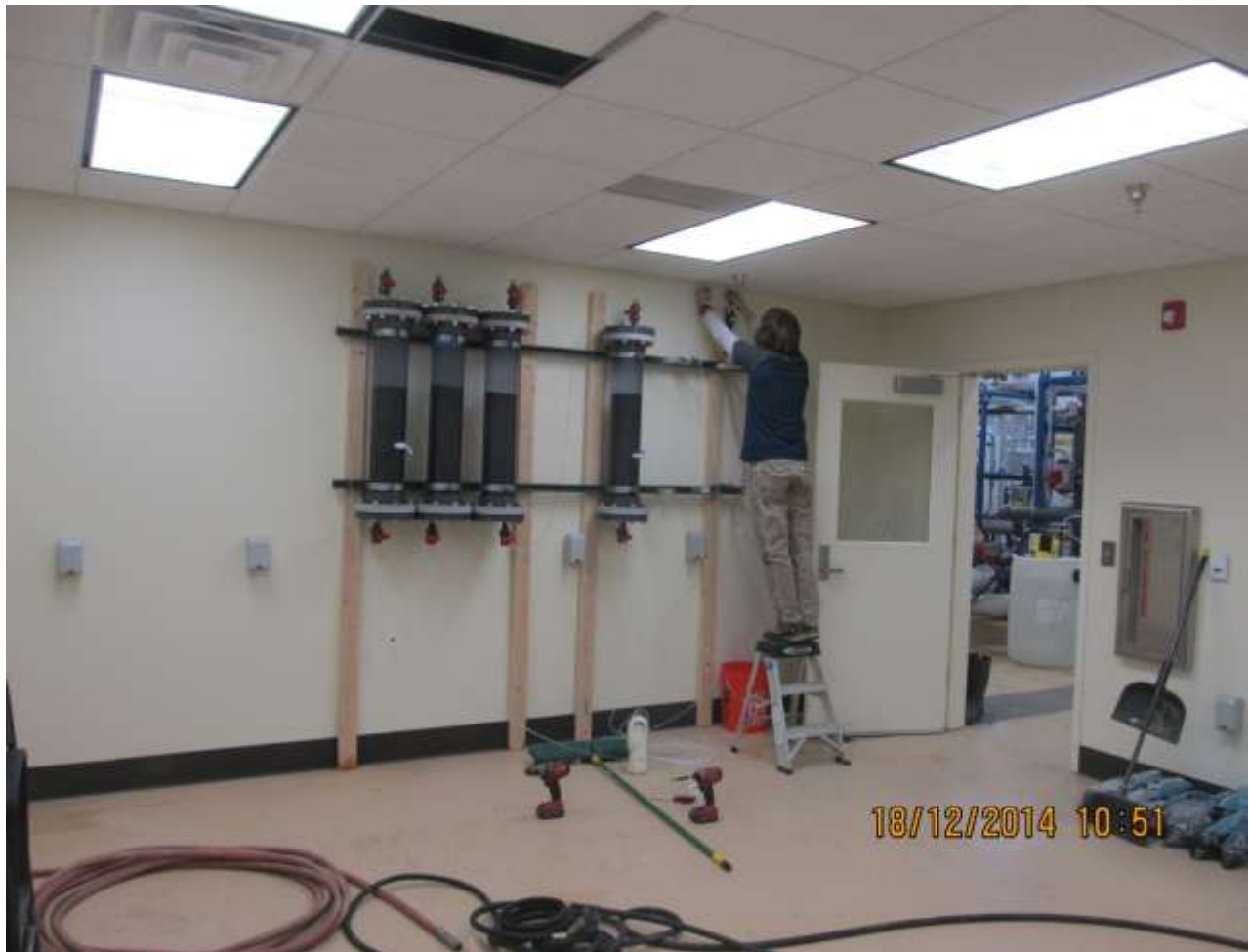
San Luis Demonstration Treatment Plant Bureau of Reclamation-Technical Service Center personnel installing apparatus for column testing in the Treatment Plant lab.
