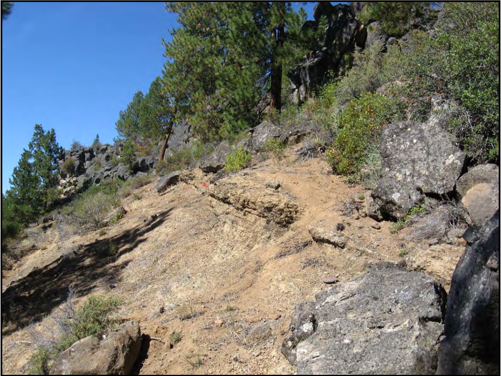
Photo 15. Close up view of upstream-dipping contact between the tuff breccia (Qt) and overlying andesite (Qa). Photo by M. McCulla, 8/22/07.
