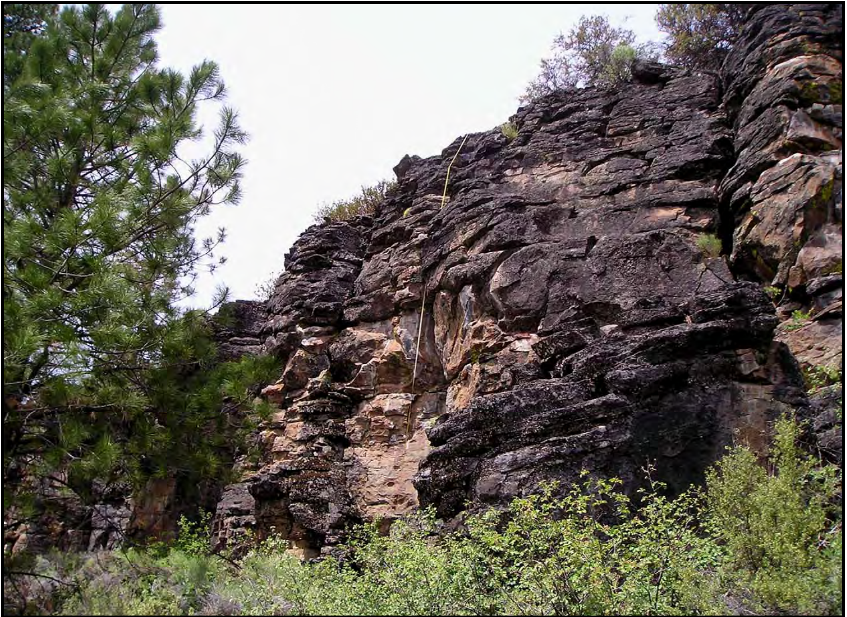
Photo 4. View of platy olivine andesite (Toa) taken from the base of Flow #1 (~el 5,010-ft.). Note the platy, sub-horizontal parting of the andesite and the widely spaced joints. Photo by M. McCulla, June 7, 2007.
