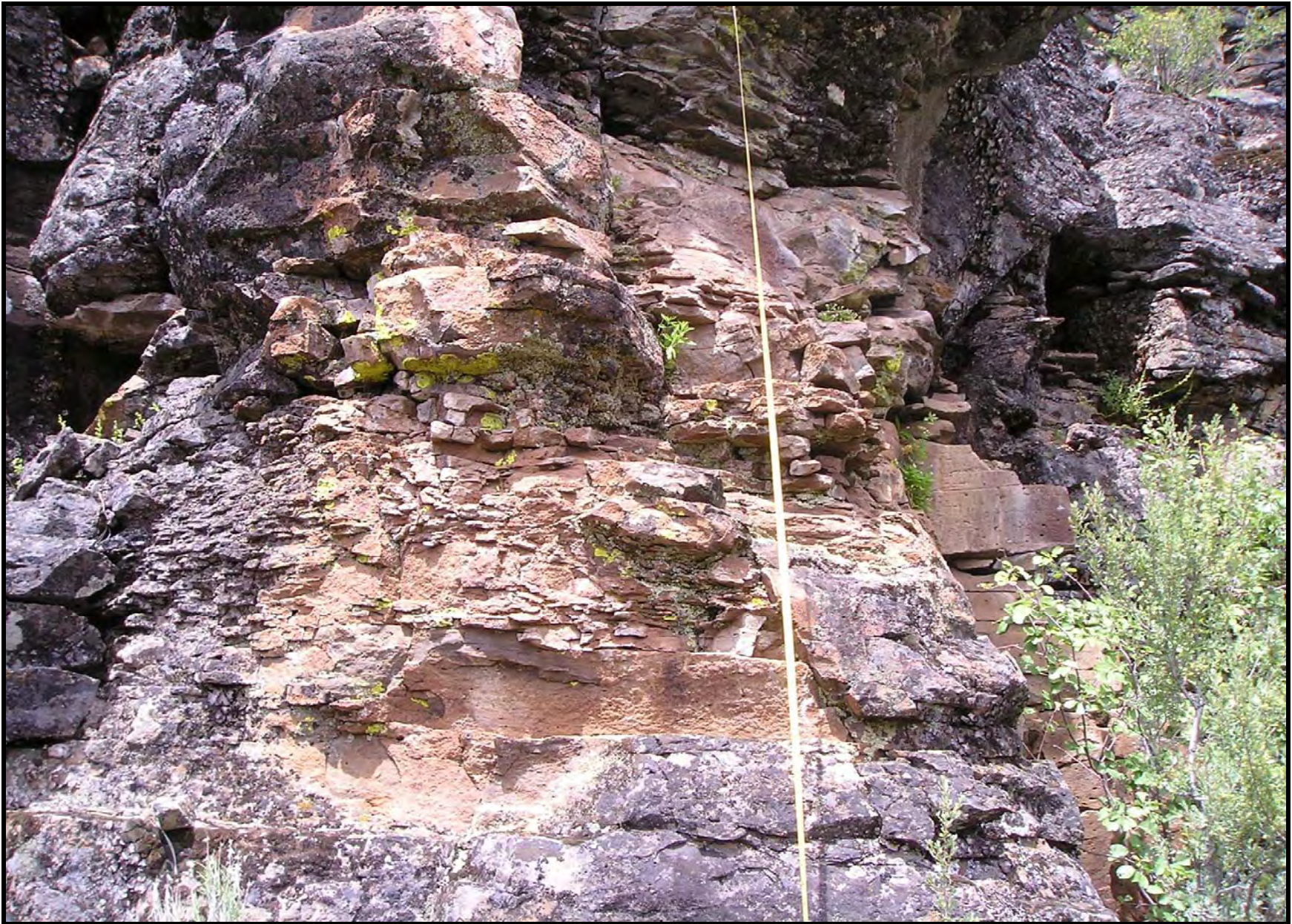
Photo 7. View of platy olivine andesite (Toa) near the base of Flow #2. Here the platy, sub-horizontal parting of the andesite is tight with few open spaces. The paucity of open spaces between plates is likely typical of the andesite with increasing depth. Photo by M. McCulla, June 7, 2007.
