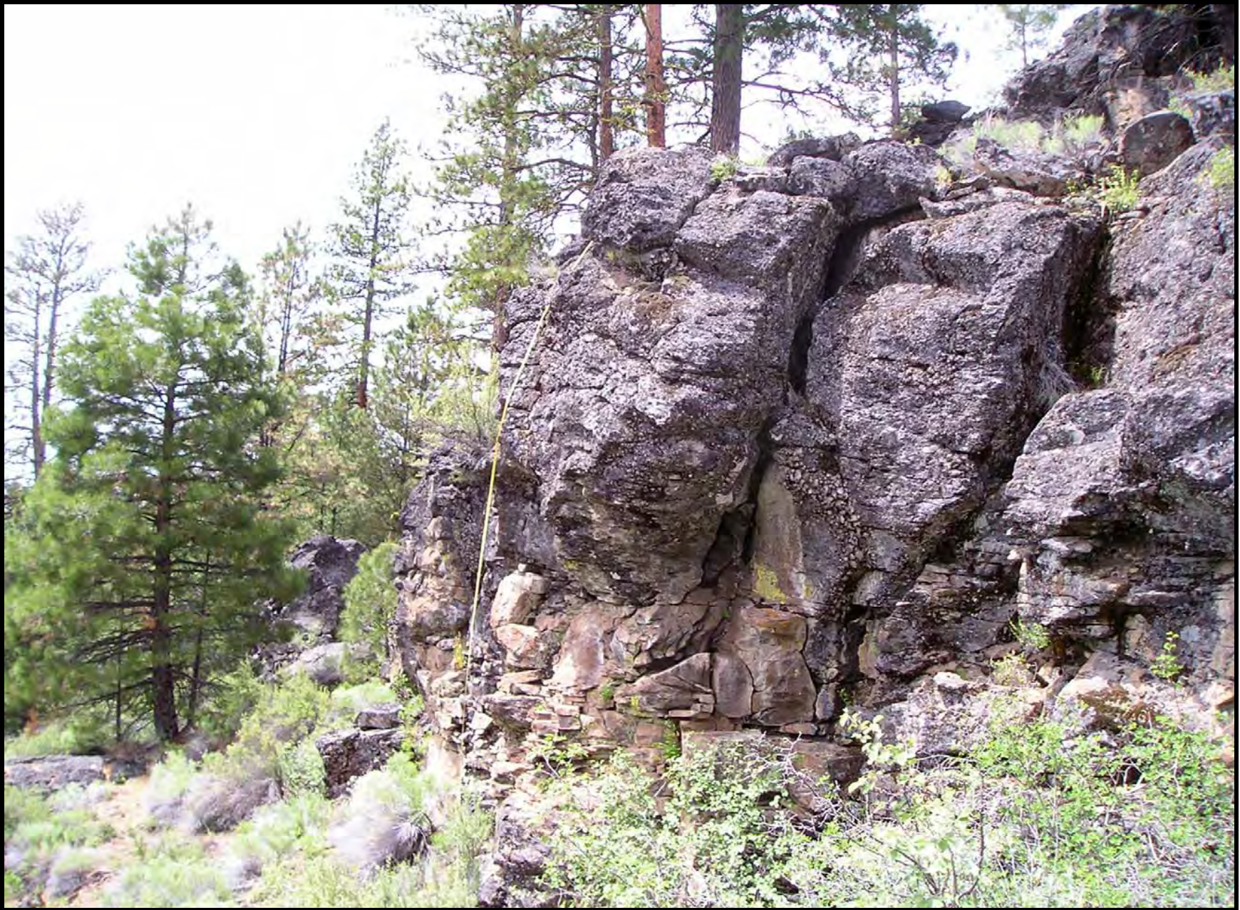
Photo 6. View of platy olivine andesite (Toa) exposed in a 21-ft. high cliff face of Flow #2. The base of the cliff is at about el 4,984 feet. Note the platy, sub-horizontal parting of the andesite and the widely spaced joints. Photo by M. McCulla, June 7, 2007.
