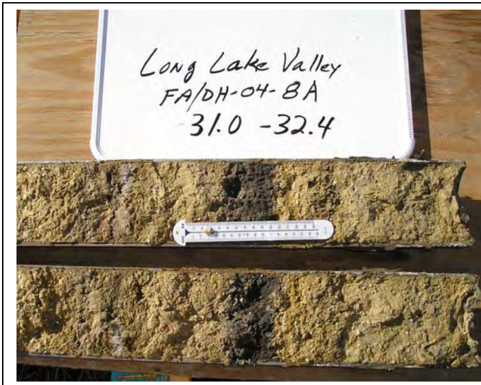
Photo 2. Very low permeability lakebed sediment (Qlb). Photo 3. Low permeability airfall tuff (Qt).
