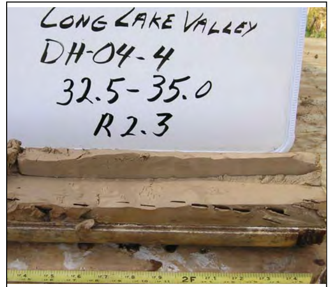
Photo 2. Very low permeability lakebed sediment (Qlb). Photo 3. Low permeability airfall tuff (Qt).
