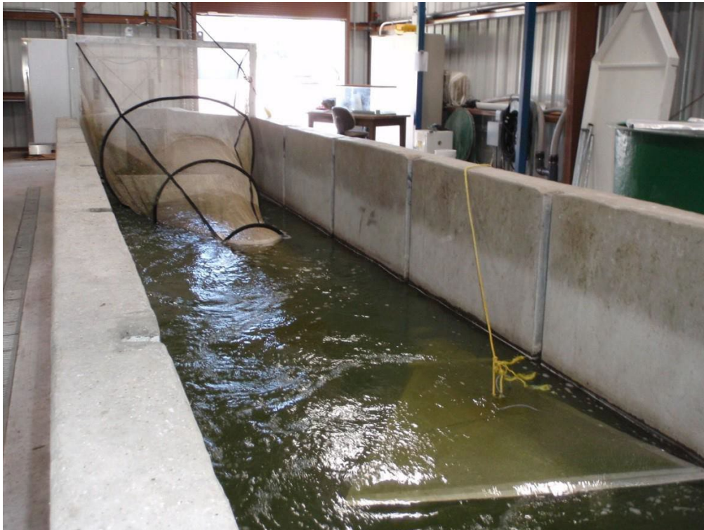
Cover Photo: Sampling flume in the Fish Evaluation Station at A Canal, Klamath Project. Photo by Darin Taylor.
