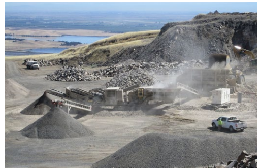
Aerial view of Basalt Hill Rock Quarry next to B.F. Sisk Dam. The front loader places excavated materials in the portable rock screening plant, that material's fed to the rock crusher, and then it is stockpiled via conveyor belts.
