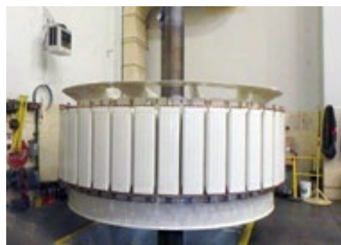
Refurbished unit rotor ready for installation; work included removal of the 40 field pole assemblies, asbestos abatement, windings’ re-insulation, amortisseur bar replacement, and refurbished pole assemblies’ re-installation.
