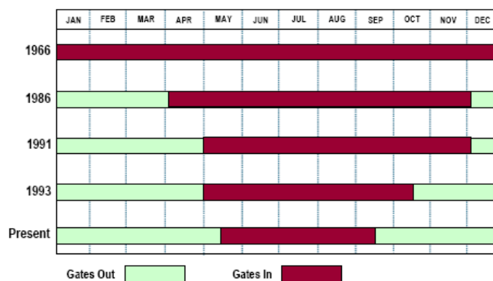
Figure 8-14. Historical patterns of gate operations at Red Bluff Diversion Dam.
