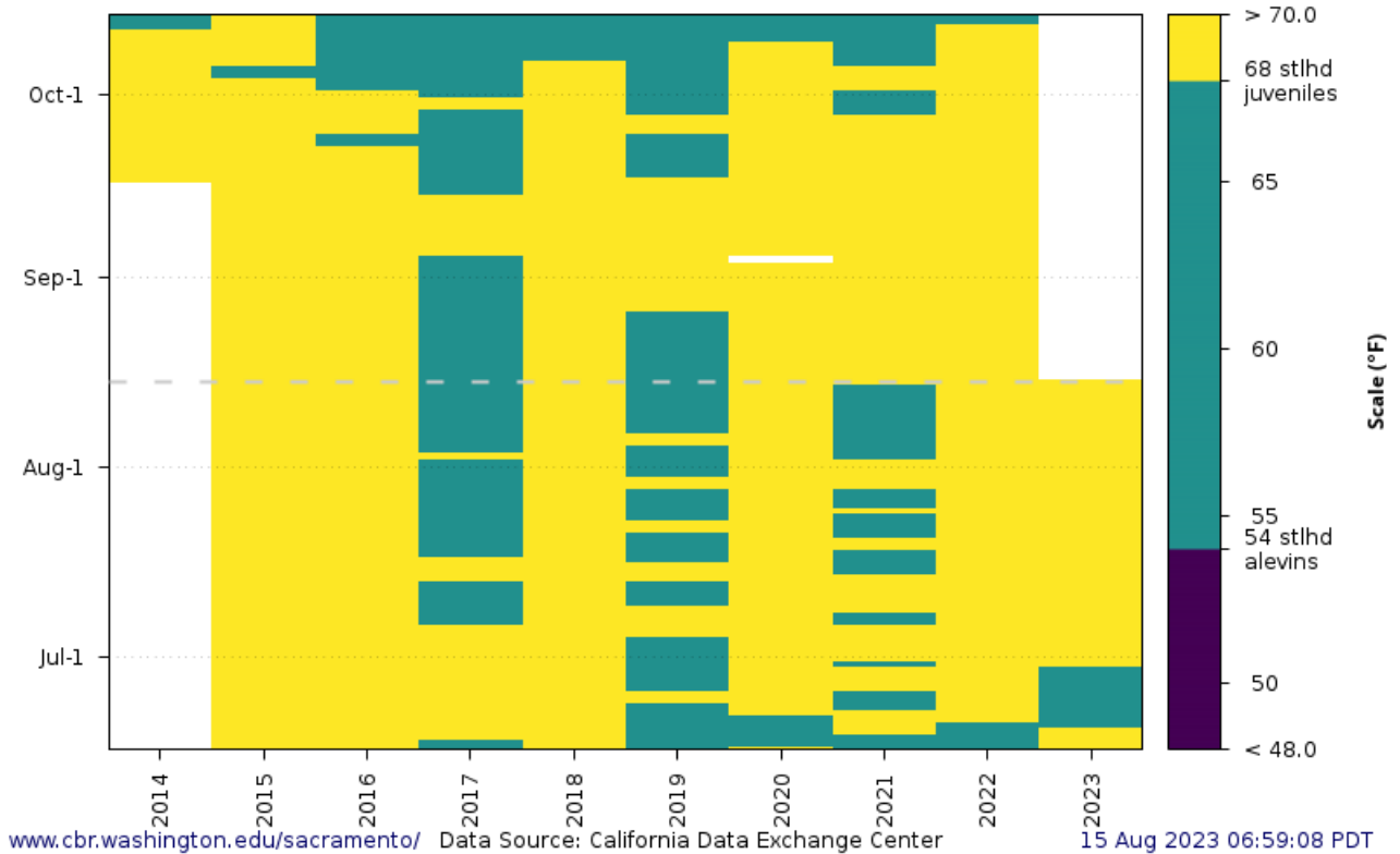
Figure 8. San Joaquin River water temperatures at Vernalis for WY 2014 to present. Figure from SacPAS using VNS station data from CDEC; temperature threshold reference line added by SWT.
