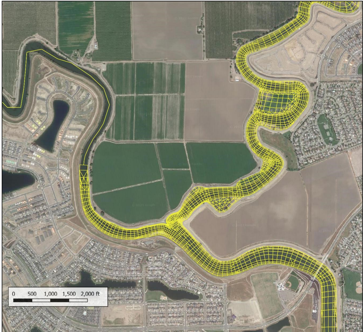
Figure 3 Baseline grid detail for the SJR scour hole project area.
