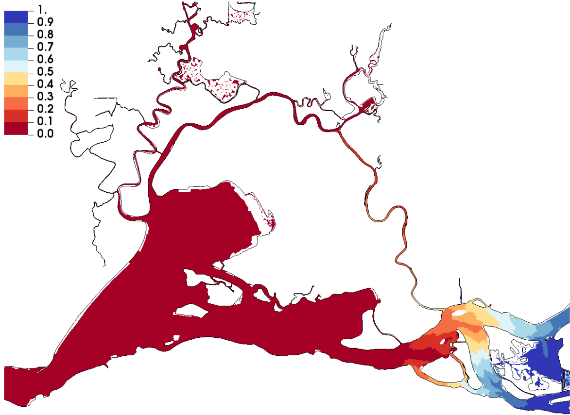
Figure 26. Fraction of time low salinity conditions were met from 9/12/21 to 9/24/21
