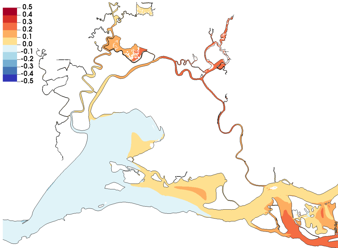
Figure 29. Change in mean salinity with and without barrier during the period August 15-28 2021, given equal hydrology
