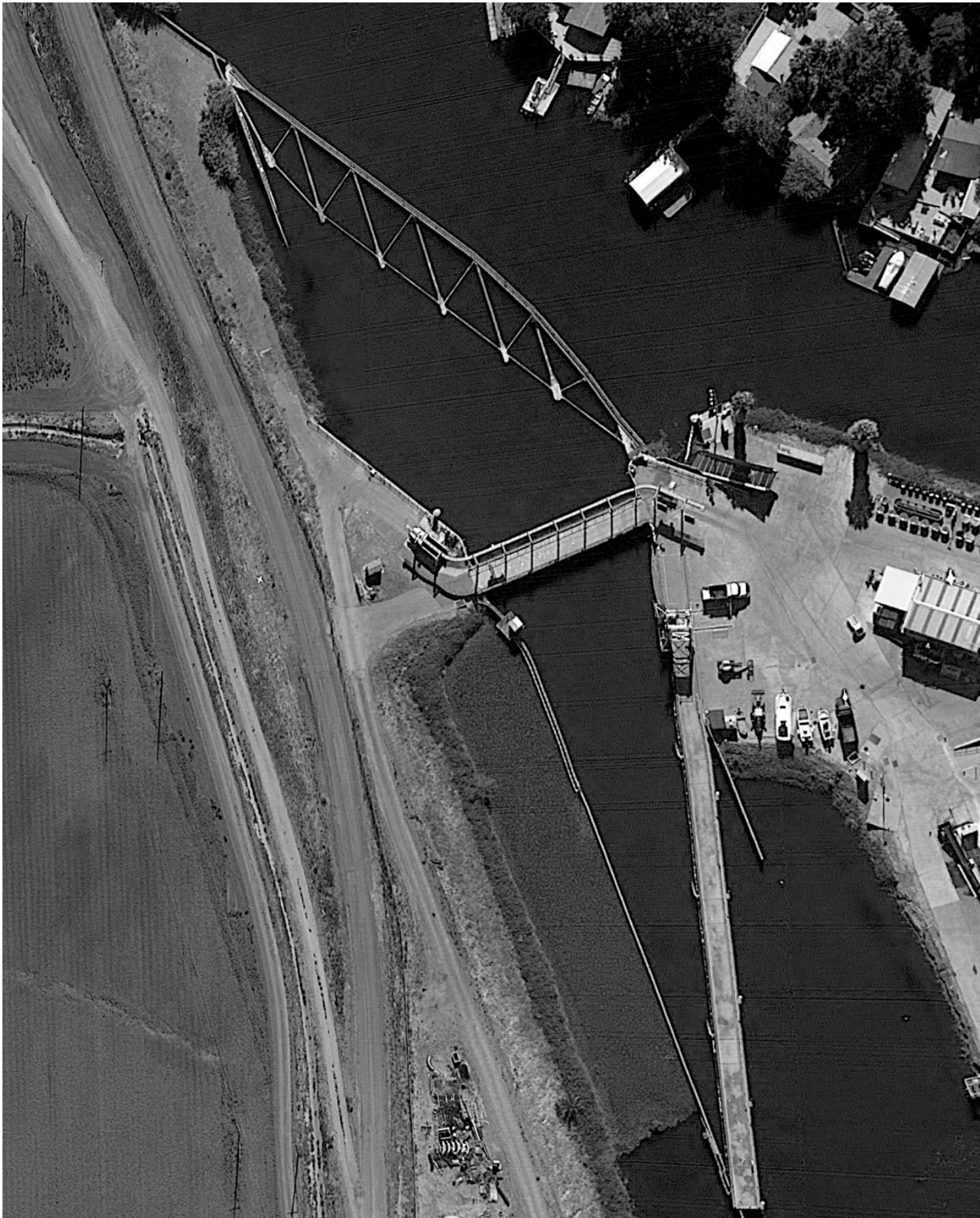
Frontispiece—Tracy Fish Collection Facility, a component of the Central Valley Project, is located in the southern region of the Sacramento-San Joaquin River Delta, about 50 miles from San Francisco, California. The facility was constructed in 1955-1956 and was designed to divert and remove fish entrained in water exported from the Delta by the C.W. “Bill” Jones Pumping Plant.
