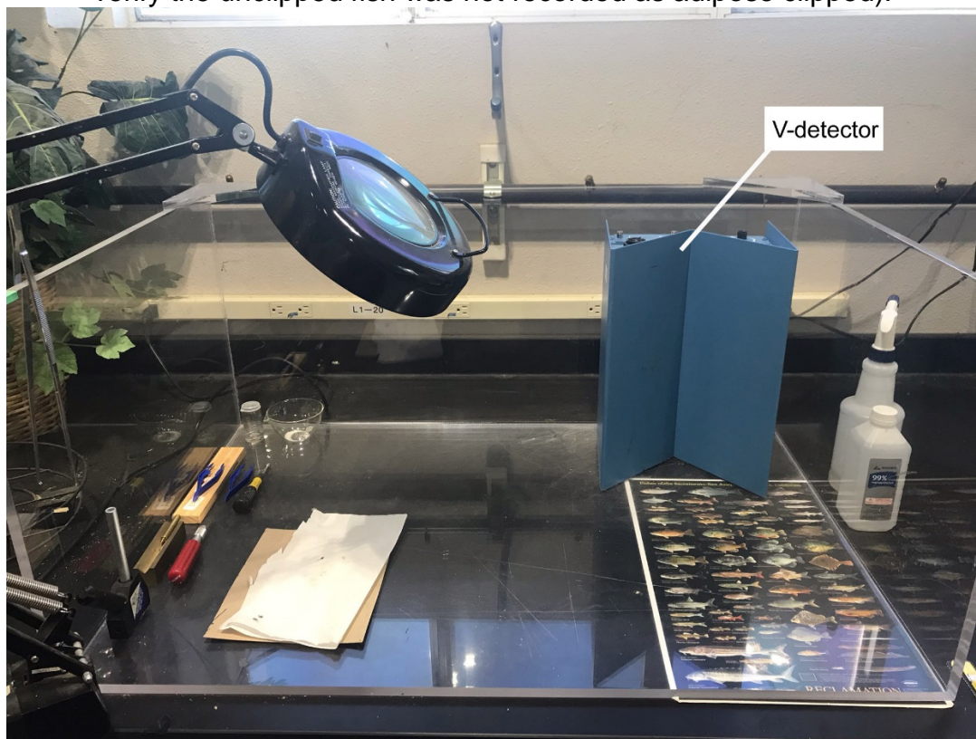
Figure 15.—Work station with a 3-side acrylic workspace, a magnifying lamp, and a tag detector called a V-detector.
