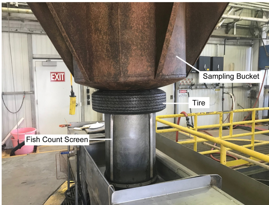
Figure 8.—Sampling bucket properly seated on the tire. There is no space between sampling bucket and the tire.
