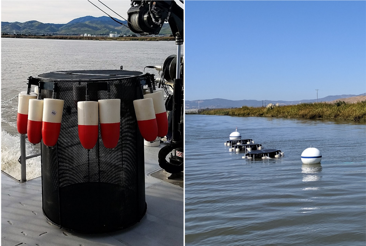
Figure 6-2. Delta Smelt Enclosure Design Used in 2019 Deployments (Photo on Left) and Three Enclosure Replicates in Suisun Marsh (Photo on Right)
