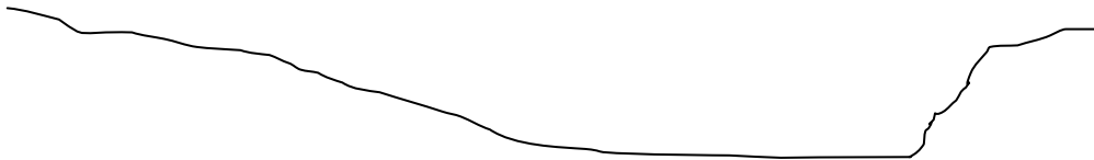
Figure A-1.—A freehand drawing of an example of a bar complex cross-section. The river is deeper on one side of the river. Generally this deeper side is on the side of the bend, and the opposite side from the bar.
