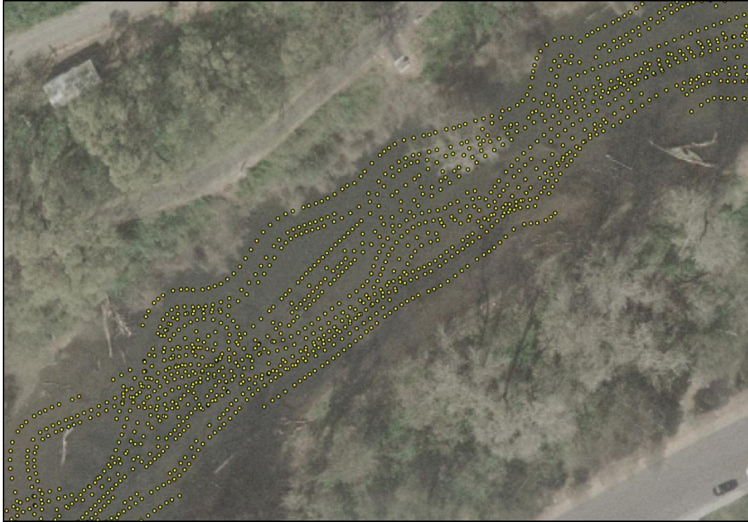
Figure E-4.—Typical survey coverage, necessarily avoiding woody debris.
