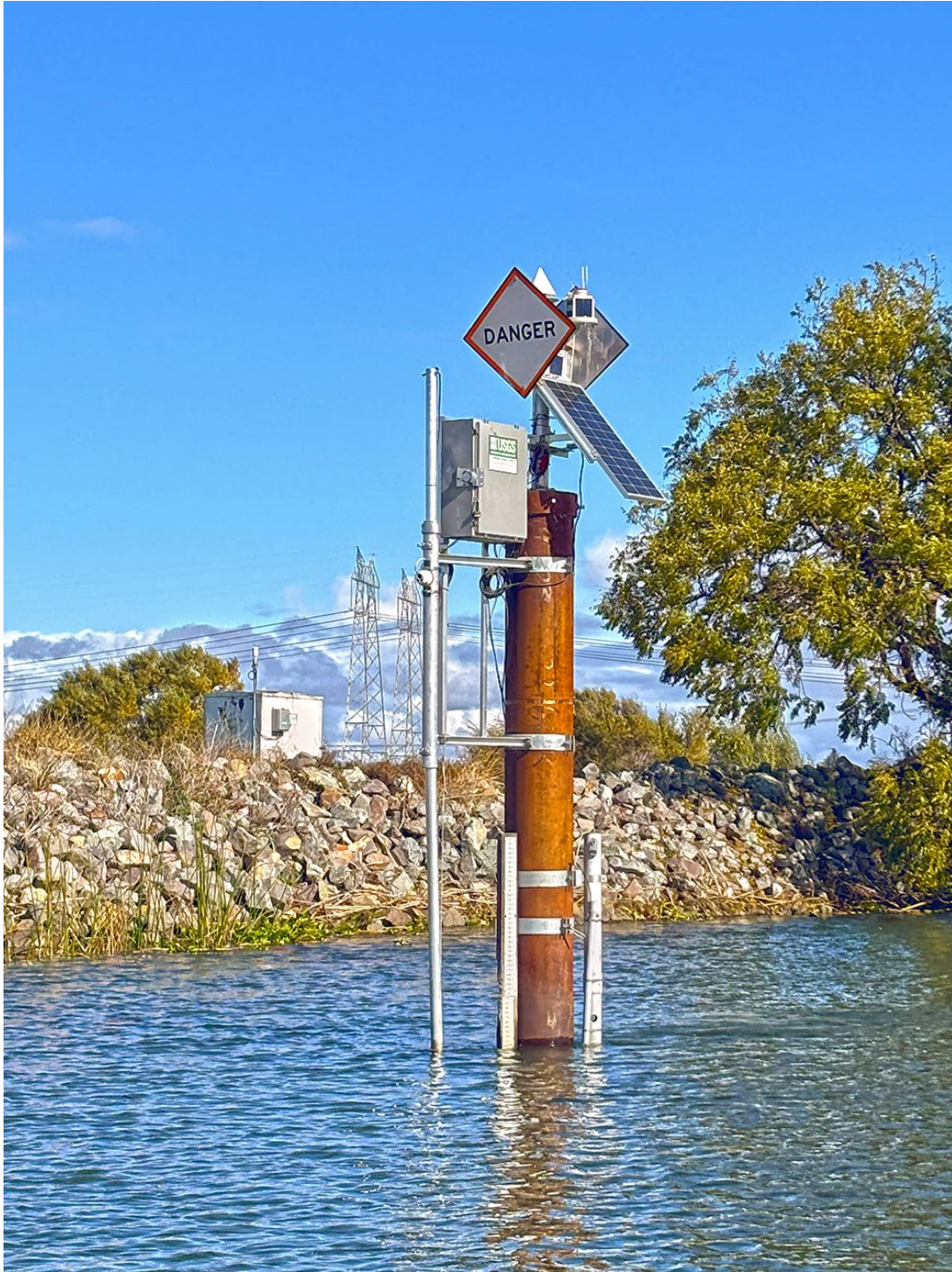
A continuous water quality monitoring station at Dutch Slough, downstream of Jersey Island in the Sacramento-San Joaquin Delta. (Lillian McCormick, Reclamation)
