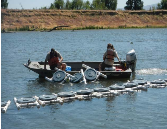
Figure 7a. A fish release at Durham Ferry. Tagged fish were held in perforated holding cans in the river for approximately 24 h after tagging. The cans were then transported to the middle of the channel approximately 200 m downstream of the holding cans where the fish were released (a).
