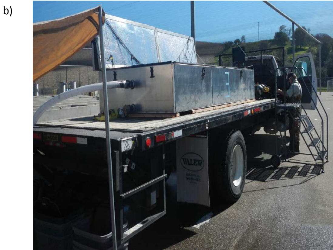
Figure 5. Dimensions and diagram of steelhead transport tanks (a) and the prepared transport truck used to transport tagged steelhead during tagging operations of the 2014 Steelhead Survival Study (b). Intake and outtake hoses provided constant flow-through of raceway water. The oxygen level of the water was monitored and adjusted as necessary during tagging and immediately before transport. Photo credits: USFWS.
