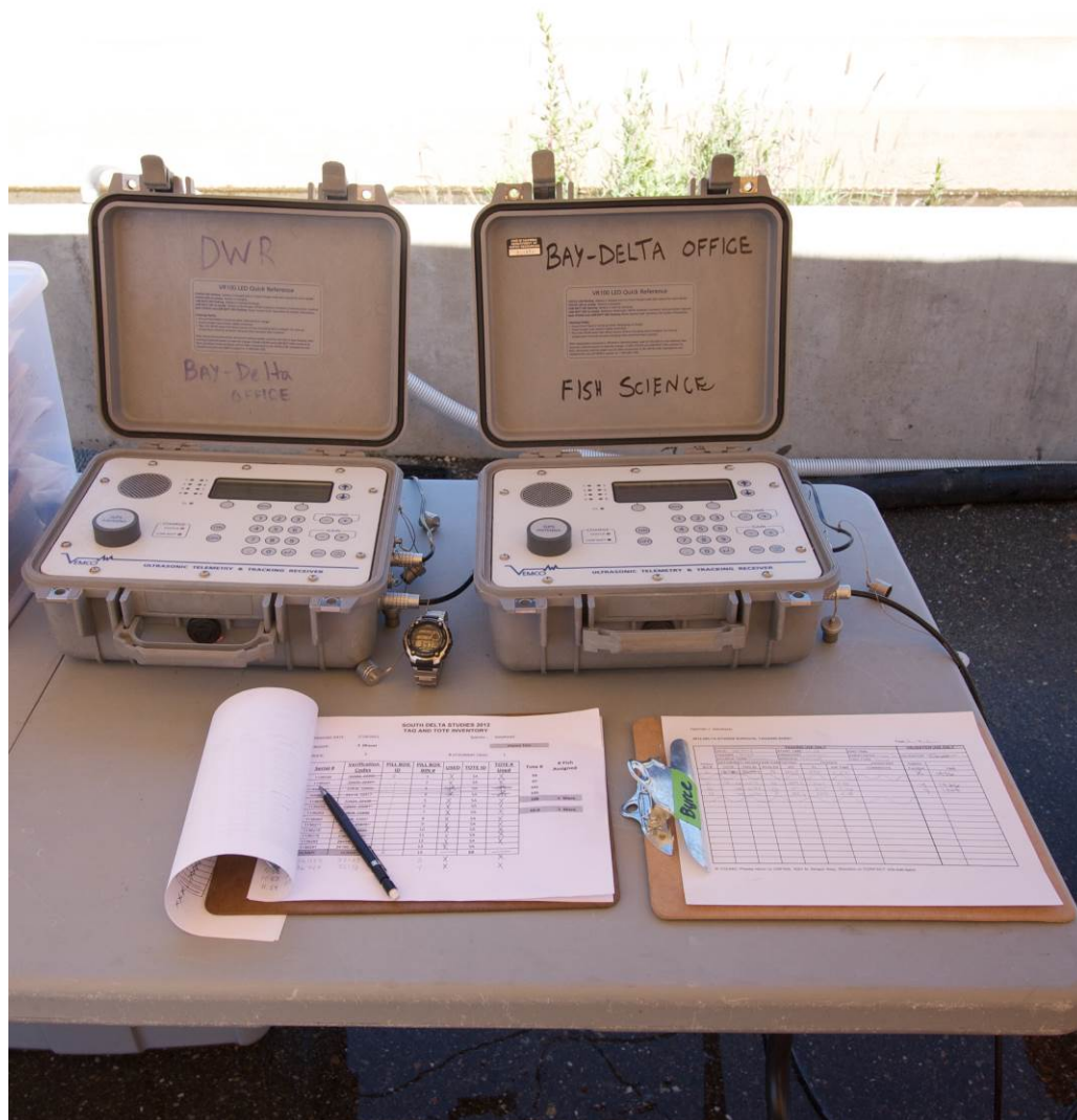
Figure 5: Two VR100 receivers for decoding tag codes from steelhead tagged with VEMCO V6 tags for the 2012 Six-Year Study. Photo Credit: Jake Osborne/USFWS
