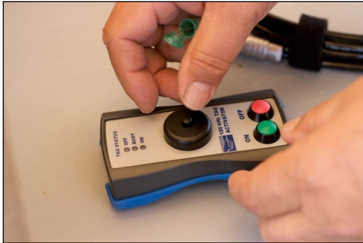
Figure 2: Tag activator for activating tags in the 2012 Six-Year Study. Photo credit: Jake Osborne/USFWS
