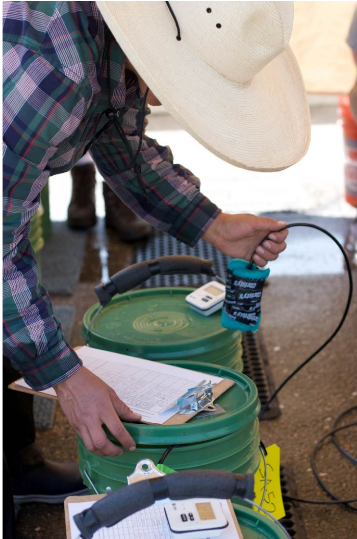
Figure 6: Hydrophone, covered with foam material to reduce multi-path electronic signal, being removed from recovery bucket after verifying tag code in tagged fish. Photo credit: Jake Osborne/USFWS
