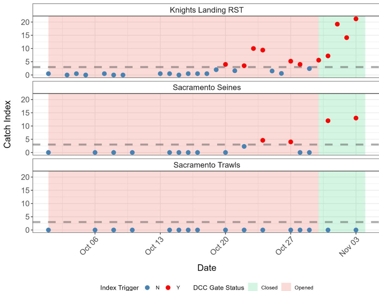
Figure 2. Summary of KLCI and SCI catch indices and DCC gate operations. Red shaded area indicates DCC gates are open, green shaded indicates closed DCC gates, the horizontal dashed line represents catch index threshold to inform DCC gate operation, blue circles represent daily catch indices below that threshold, and red circles indicate daily catch indices that exceed that threshold.
