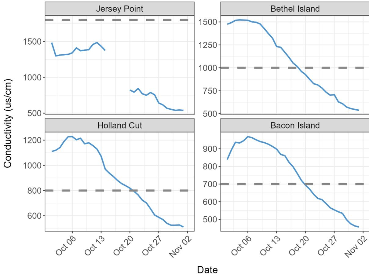
Figure 4. Conductivity (umhos/cm) at Jersey Point, Bethel Island, Holland Cut, and Bacon Island with associated standards thresholds (horizontal dashed line).
