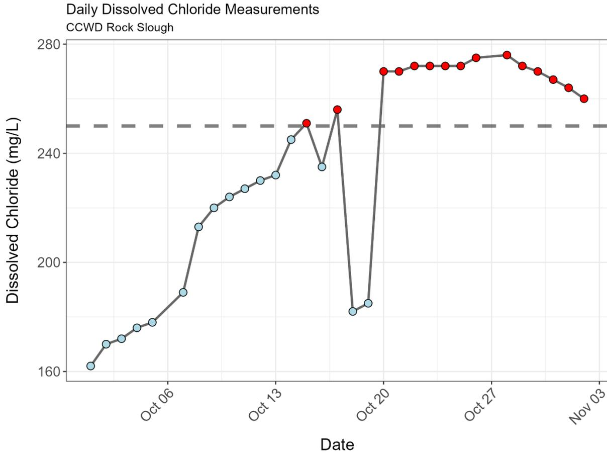
Figure 5. Dissolved Chloride (mg/L) measured at Rock Slough Pumping Plant intake. Red circles indicate exceedance of d-1641 Dissolved Chloride standard of 250 mg/L.
