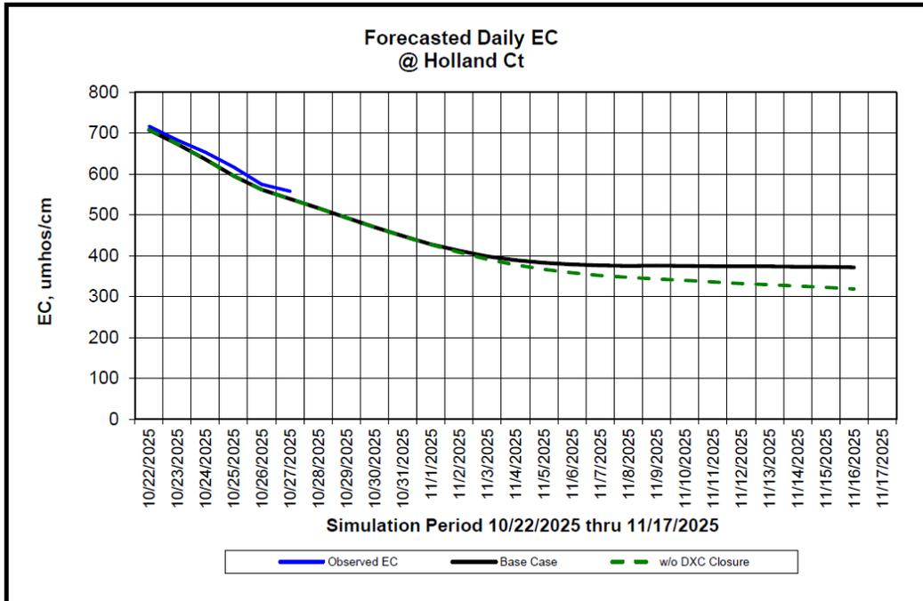
Figure 8. DSM2 EC modeling at Holland Cut. Water quality concern level is 800 umhos/cm. Updated 10/28/25.
